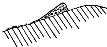
FIG. 39.—Diagrammatic cross-section of the marginal ridge as it occurs on the south slope of the Devil's Nose. The slope below, though glaciated, is nearly free from drift.
