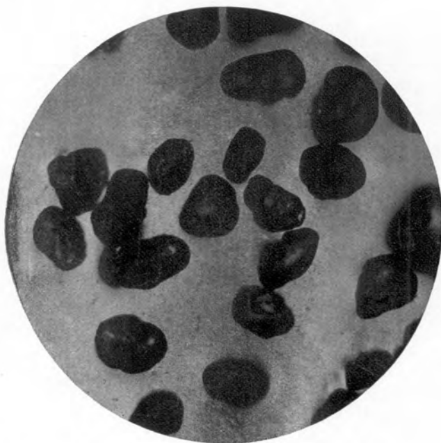
Fig. 2. Same locality. Grains retained on 40 mesh. \times 18 . By transmitted light.
