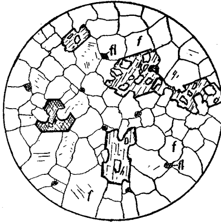
FIG. 9.—Skeleton crystals of amphibole in syenite. h, Amphibole. b, Feldspar. fl, Fluorite.
