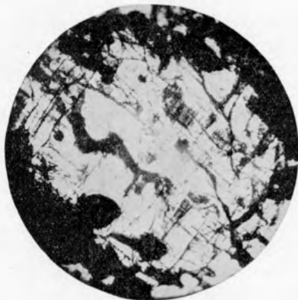
FIG. 10.—Photomicrograph of fayalite in nepheline syenite; \times 60 . The fayalite, light-colored, is surrounded on nearly all sides by a black border of magnetic iron oxide. Portions of it are in contact with feldspar and hedenbergite. The greatest length of the fayalite in this section is along the c axis, parallel to which is indistinct parting or cleavage.
