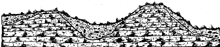
FIG. 18. Diagrammatic section showing relation of drift to underlying rock where the drift is thin relative to the relief of the underlying rock.
