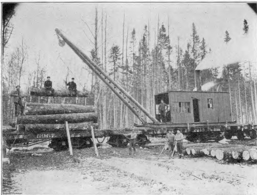
A. STEAM LOG LOADER. CAPACITY 15 CARS PER DAY.
