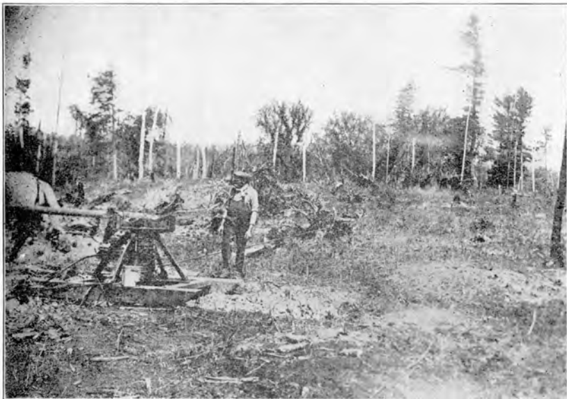
FIG. 1. A CHEAP BUT SATISFACTORY STUMP PULLER.
