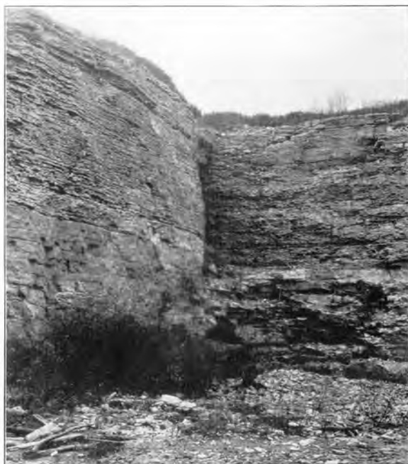
The Columbus city quarry. The rock is the Trenton limestone, soft, thin-bedded, and of inferior quality for road making. The position of the quarry faces is controlled by vertical fissures (joint planes) which cut the rock into rectangular blocks.
