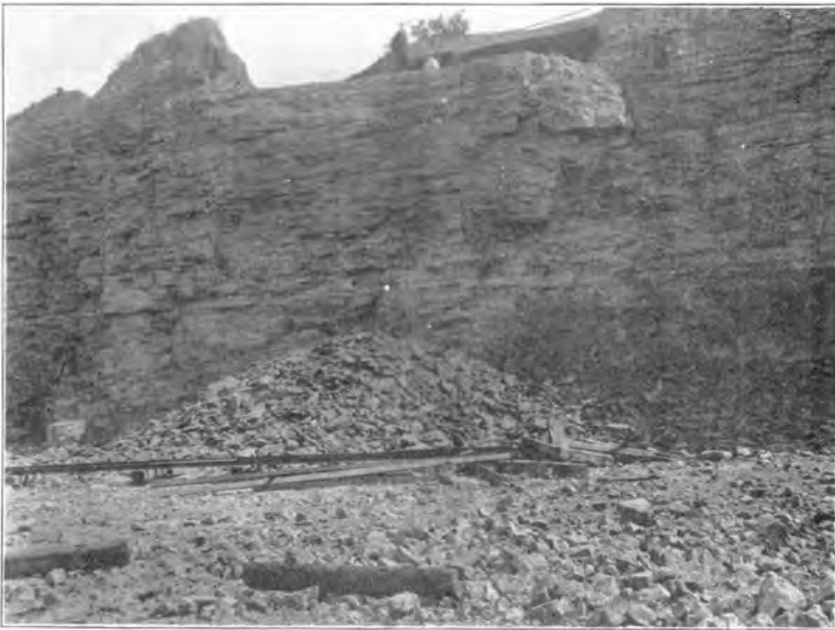
The Andrew Barnes quarry at Janesville. The rock is Trenton limestone. It is of uniform quality for road construction. Although not as good a road material as the best grades of Niagara limestone from the eastern part of the state, it is very satisfactory for local purposes.
