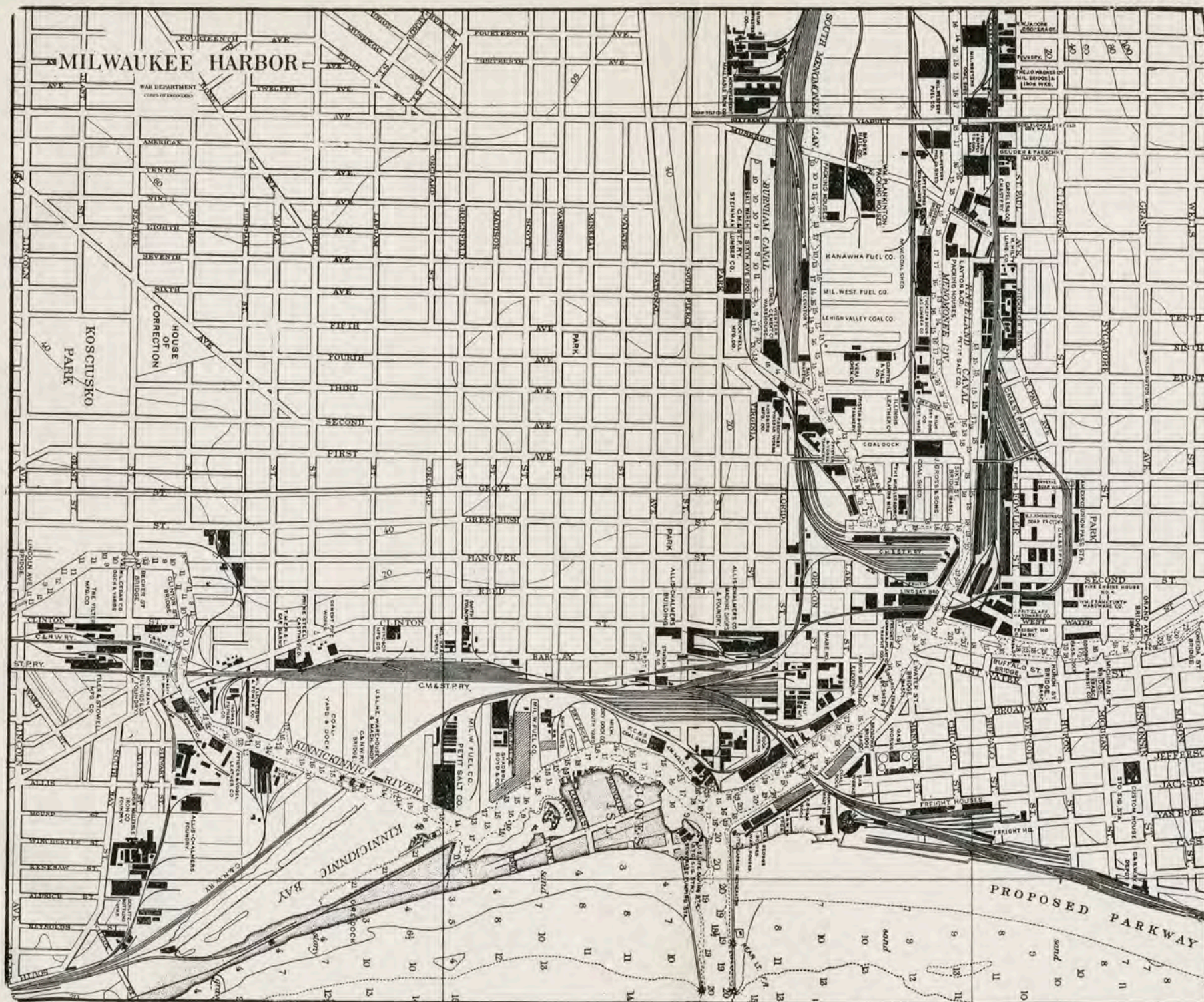
Map of a part of Milwaukee. Numbers in the rivers and lake indicate depth of the water in feet. Note that the railways and their freight yards, the warehouses, and coal yards are all near the waterways. (Map from U. S. Dept. of Commerce, Miscel. Series No. 33, 1916)
