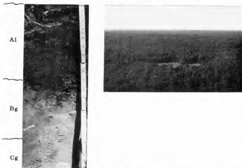
Figure 21. The soil profile (left) is of a poorly drained marsh border soil called Humic-Gley (Aquoll). There are two major horizons: the thick black A1 (0 to 10 inches) and the bluish-gray Bg horizon (10 to 17 inches). The landscape shows a treeless bog bordered by Humic-Gley soil (unit 25 on the soil map).
