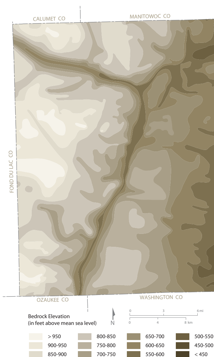
Figure 3. Bedrock topographic map of Sheboygan County, contour interval 100 ft (30 m). The bedrock surface slopes to the east with a deep valley cutting down the center.
