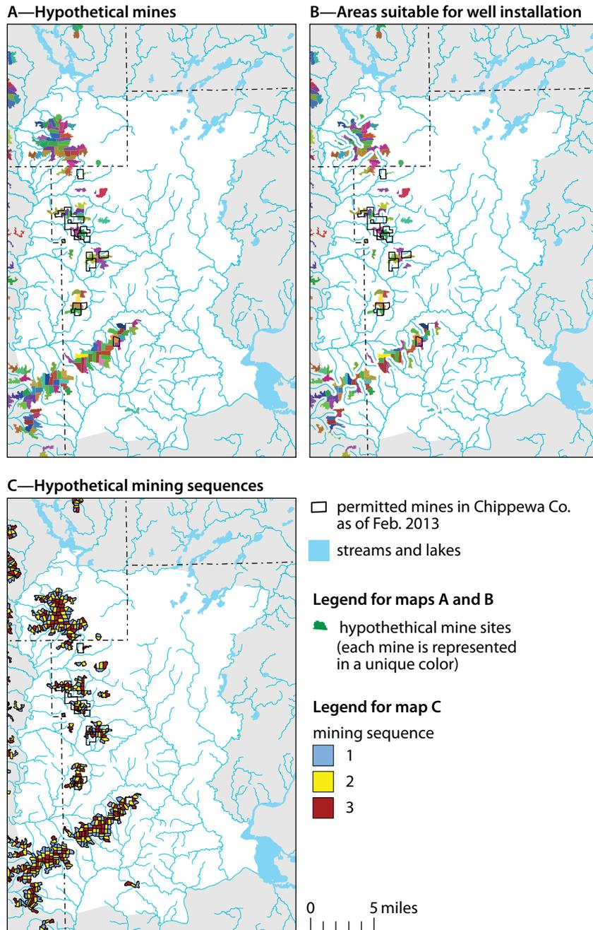
**Figure 34.** Mine buildout maps showing (A) the minable Wonevoc resource segmented into 155 hypothetical mines of approximately 150 minable acres each, (B) segments with well locations at least 1,200 feet from a stream, and (C) hypothetical three-step mine development sequences.
