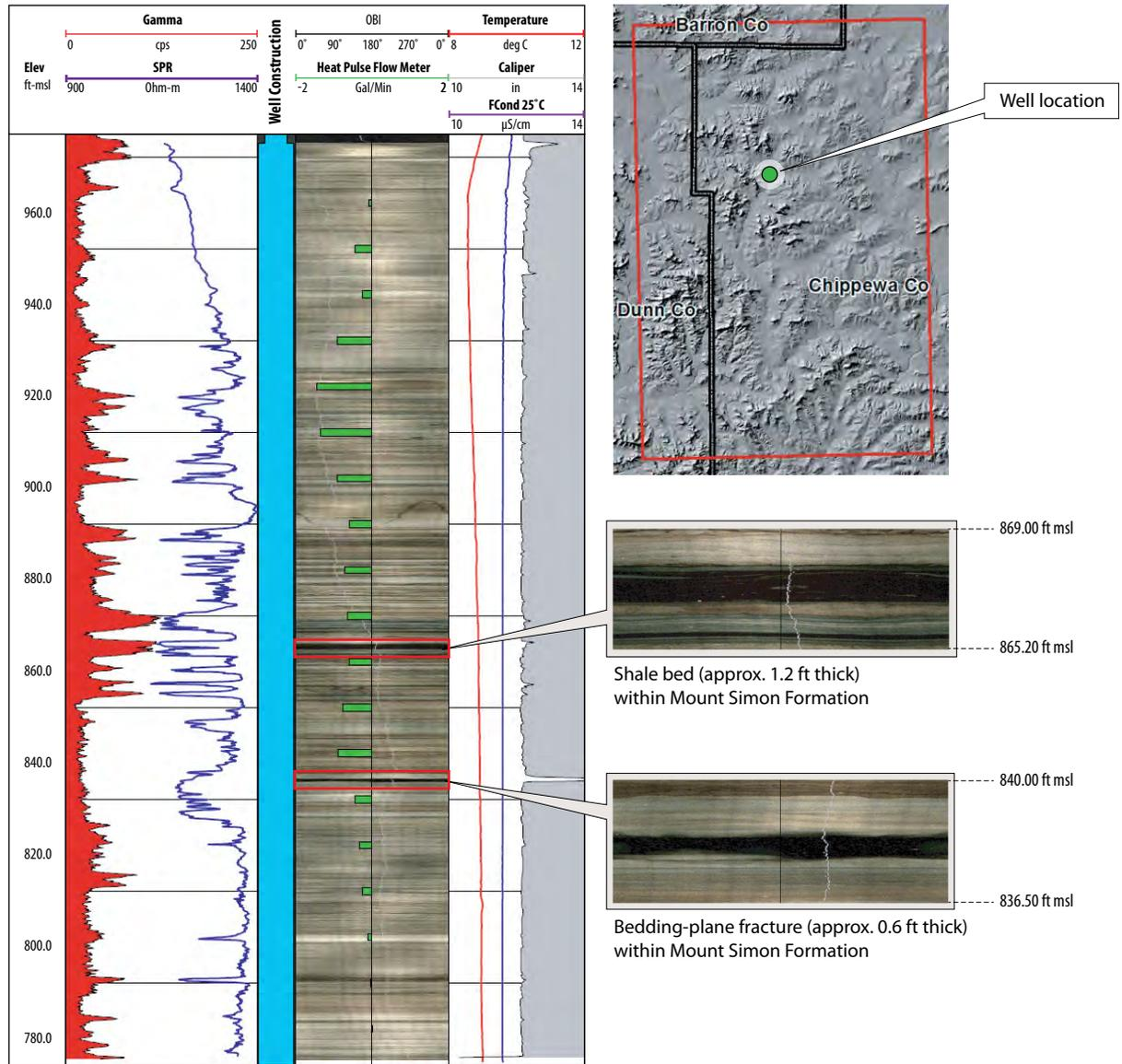
**Figure 2.** Example borehole geophysical log. High-resolution imagery from the optical borehole imaging (OBI) tool reveals a shale bed and a bedding-plane fracture within the Mount Simon Formation. From the Superior Silica Sands Culver mine (WGNHS ID 9000341).
