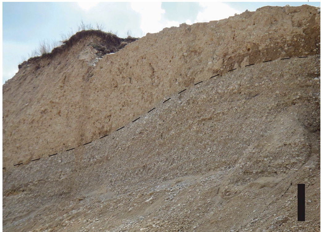
Figure 10. Vertical wall of gravel pit in drumlin located in Fond du Lac County. Wall is about 8.3 m high and exposes gravelly meltwater-stream sediment beneath till of the Horicon Member. Dashed line shows the contact between the two sedimentary units. Scale bar is approximately 1 m.
