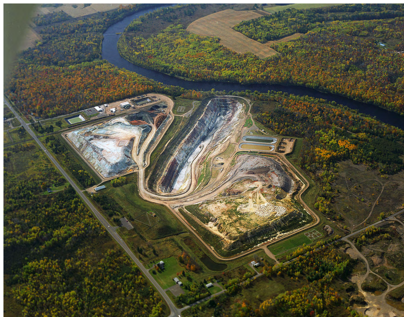
▲ Flambeau mine, 1996: Production at the Flambeau mine began in 1993. The mine produced 1.9 million tons of high-grade copper ore—yielding 181,000 tons of copper, 3.3 million ounces of silver, and 334,000 ounces of gold—before it was closed in 1997.
