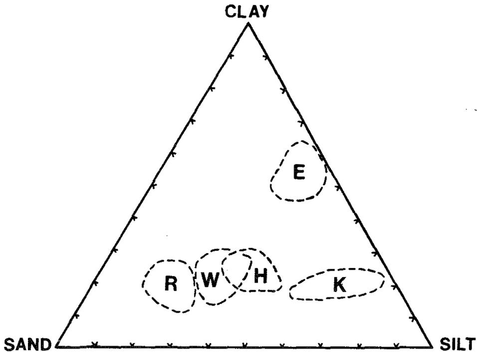
Figure 1.--Ternary diagram illustrating C-horizon textures of the pre-Wisconsinan units in west-central Wisconsin. Enclosed areas show distribution of (R) 23 samples of River Falls Formation, (W) 10 samples of Woodville Member, (H) 26 samples kinnick Member, and (E) 7 samples of Eau Galle Member.
