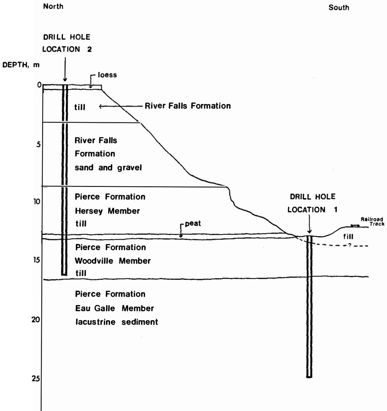
Figure 10.--Cross section of the Woodville railroad cut.
