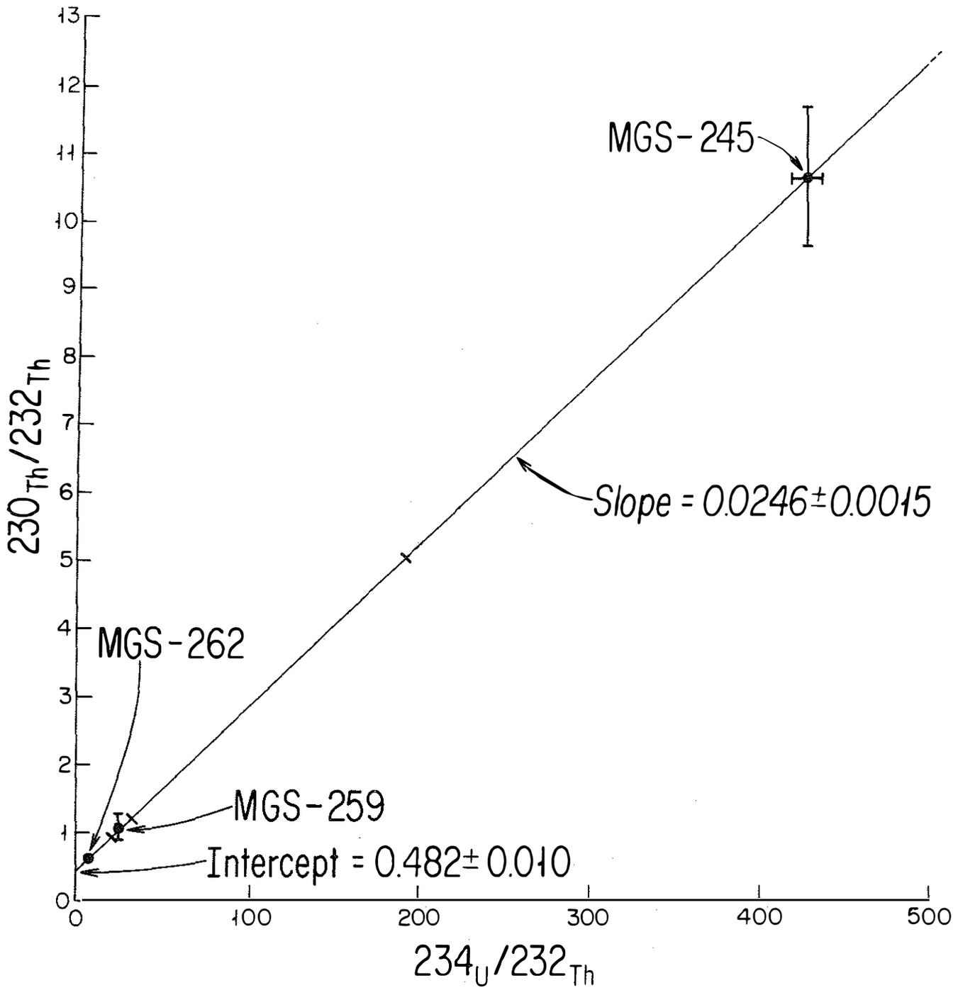
Figure 1.--Isochron plot of uranium and thorium activity-ratio data from Taylors Falls cemented gravel.
