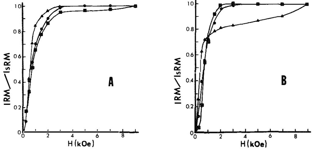
Figure 4.--Isothermal-remanence acquisition curves for representative samples from (A) the Kinnickinnic Member (lacustrine sediments) and (B) the tills of the Hersey Member (square and triangular symbols) and the River Falls Formation (dots). IRM is the isothermal remanent magnetization, IsRM is the isothermal saturation remanent magnetization, and H is the magnetic field intensity (1 Oe=76.6 ampere/meter).
