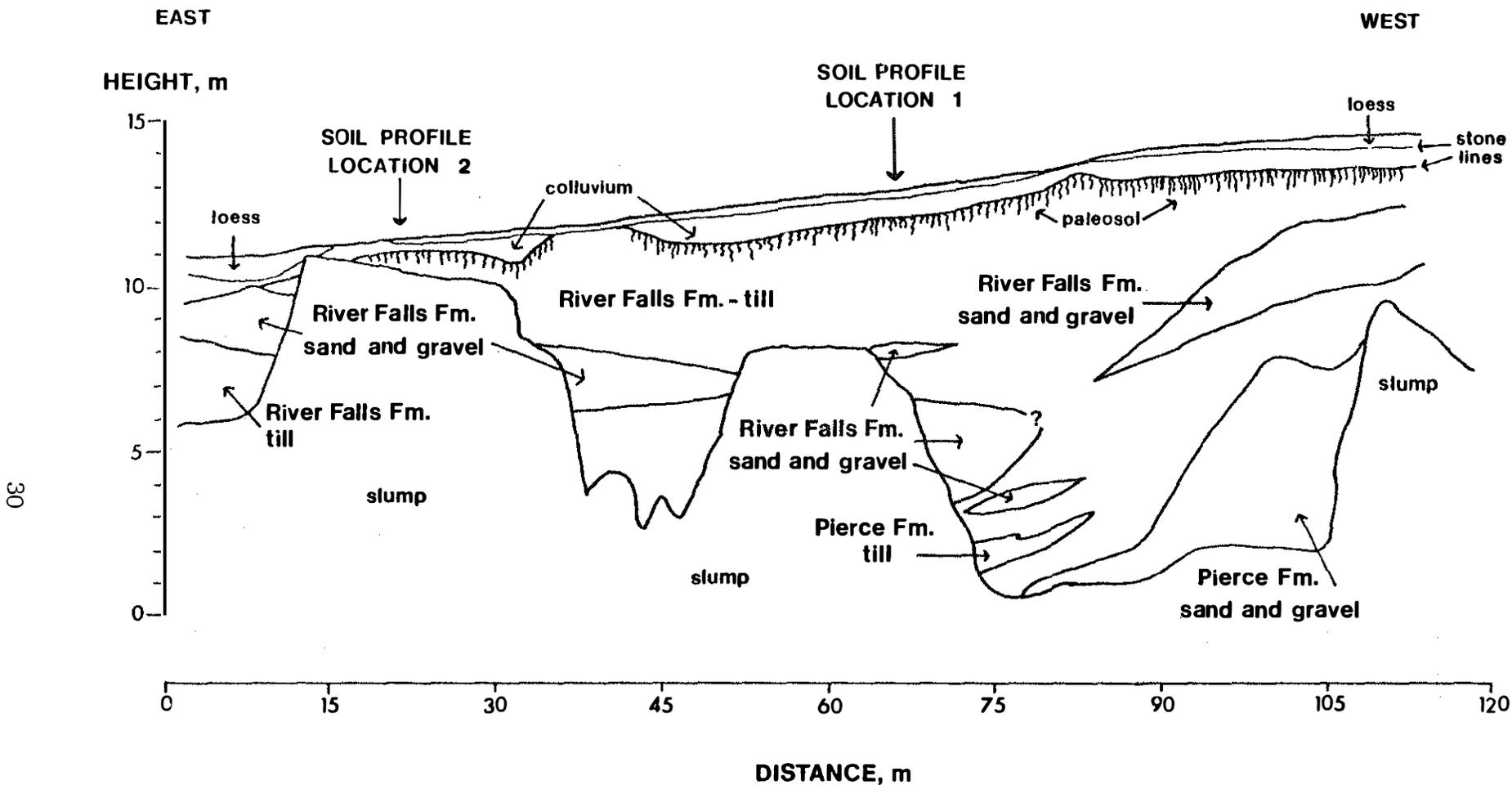
Figure 7.--Cross section of the southeast wall of the County Highway E gravel quarry in the River Falls Formation.
