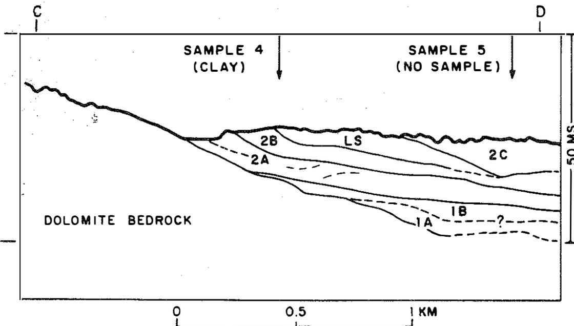
FIGURE 6.--Acoustic profile and interpretation along C-D of figure 5. The sub-units of till were identified by extrapolating to their outcrops in the nearshore bluffs except for till units 1A and 1B which do not outcrop, but lie roughly 7 m below the lake bottom at the location of sample 4.
