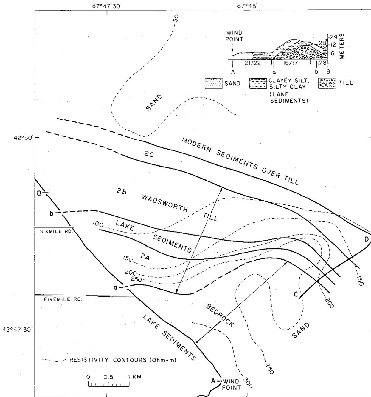
FIGURE 5.--Interpretation north of Wind Point. Because of erosion, till units are exposed on the lake floor and can be traced to shore, where they can be identified. A gravel lag overlies most of the area surveyed. High resistivity measured near Wind Point reflects the rock outcrop. Dotted lines are iso-resistivity contours.
