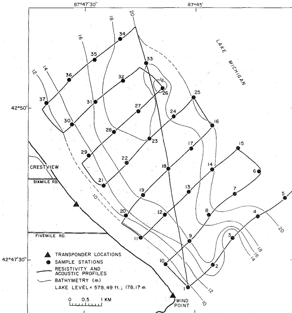
FIGURE 4.--Bathymetry based upon the 1977 acoustic profiles north of Wind Point. Sample station locations are also shown.
