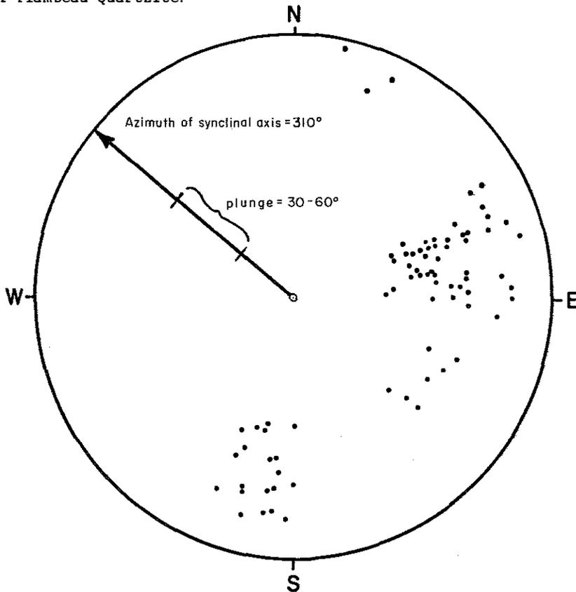
Figure 3.--Poles to bedding plotted with inferred axis and plunge of syncline (80 measurements).
