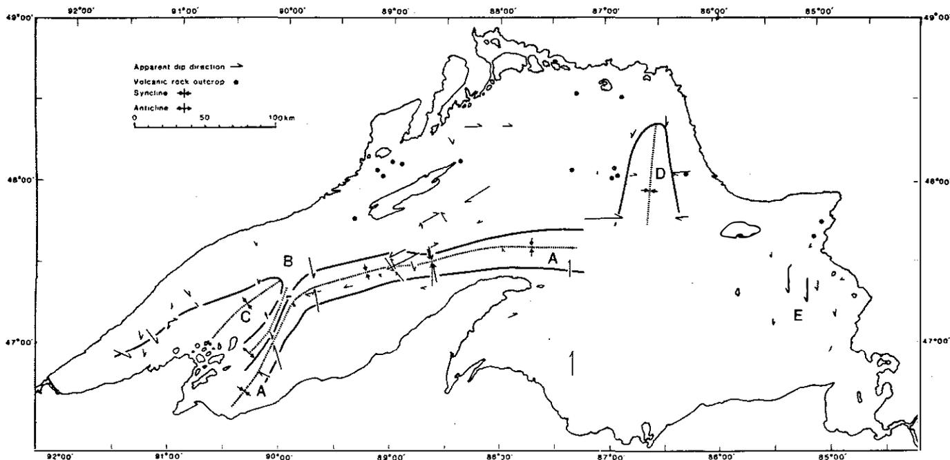
Figure 4. Apparent dip directions to subcrops observed on seismic-reflection profiles. A = Lake Superior depositional syncline; B = Anticline; C = southwest-plunging syncline; D = south-plunging syncline; E = south apparent dips. (from Wold and others, 1982).
