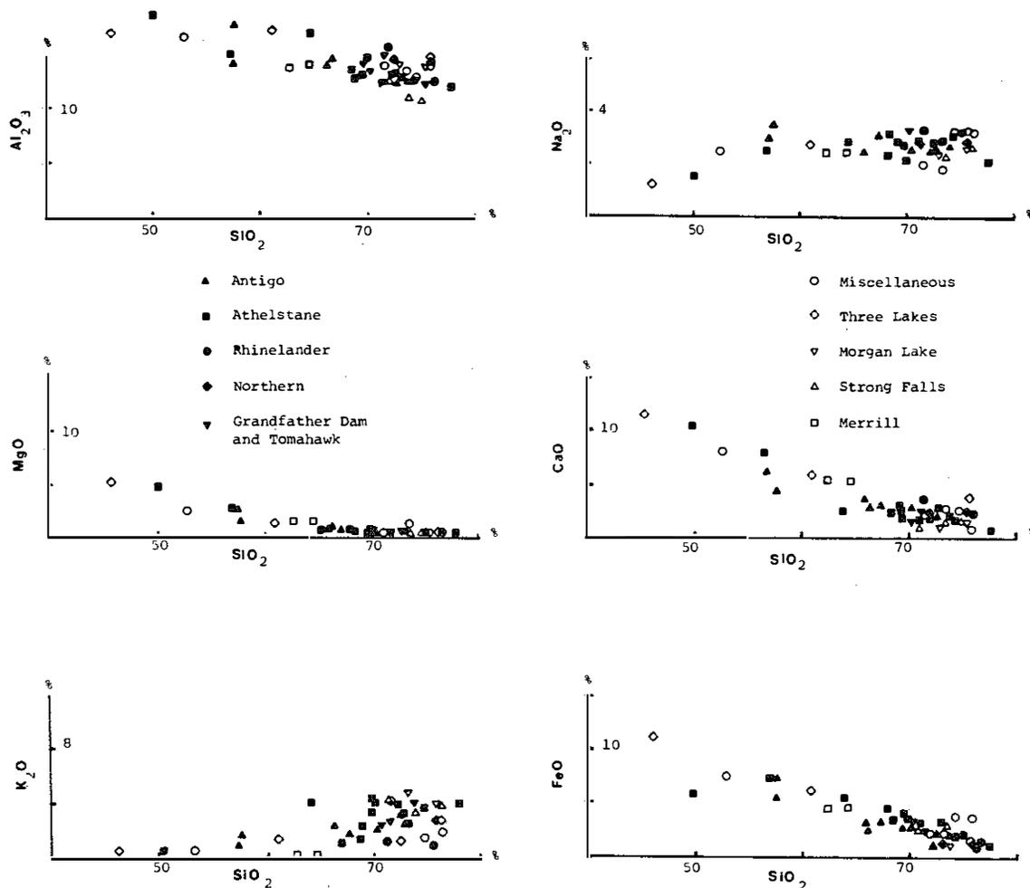
Figure 5. Harker variation diagrams for granitic rock from northeastern Wisconsin.
