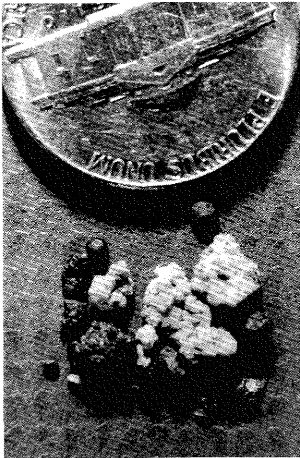
Figure 8. Oolitic hematite and oolitic dolomite, from a sample interval including Maquoketa shale and Silurian dolomite from a well in sec. 31, T. 9 N., R. 14 E. Otoe County, Nebraska.
