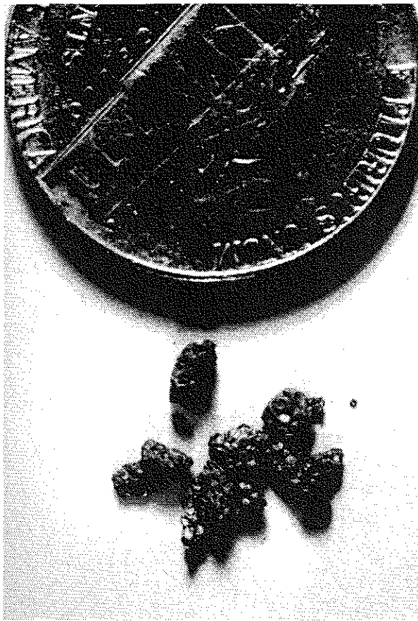
Figure 3. Oolitic hematite in the Maquoketa shale from a well in sec., 14 T. 1 N., R. 16 E. Richardson County, Nebraska.
