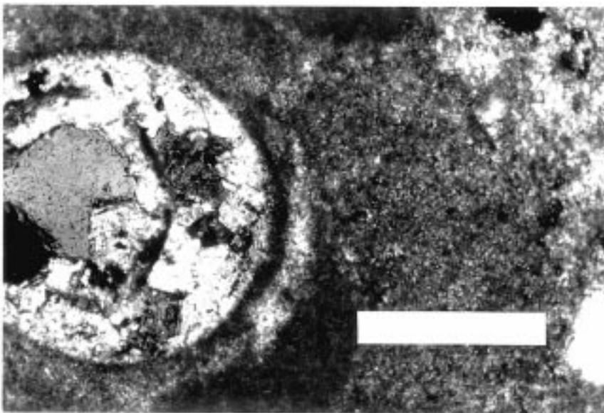
**Figure 6.** Dolomitized ooid within dolomitized peloidal packstone-wackestone matrix, from lower Oneota Formation at Madison, Wisconsin. Note relatively coarse dolomite crystals within ooid (left) and finer dolomite crystals within micritic-textured peloidal packstone-wackestone (right). Ooid core is a grain of quartz silt. Scale bar = 0.2 mm.
