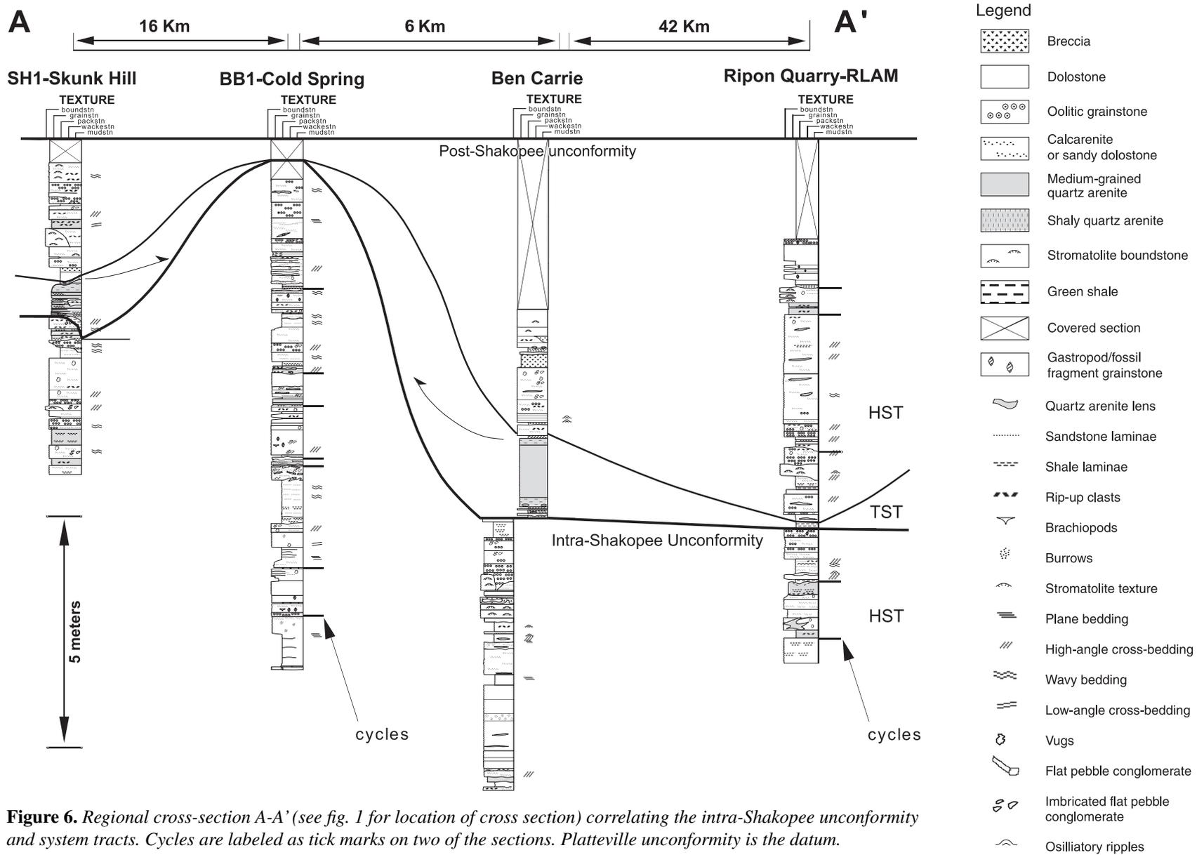
**Figure 6.** Regional cross-section A-A' (see fig. 1 for location of cross section) correlating the intra-Shakopee unconformity and system tracts. Cycles are labeled as tick marks on two of the sections. Platteville unconformity is the datum.
