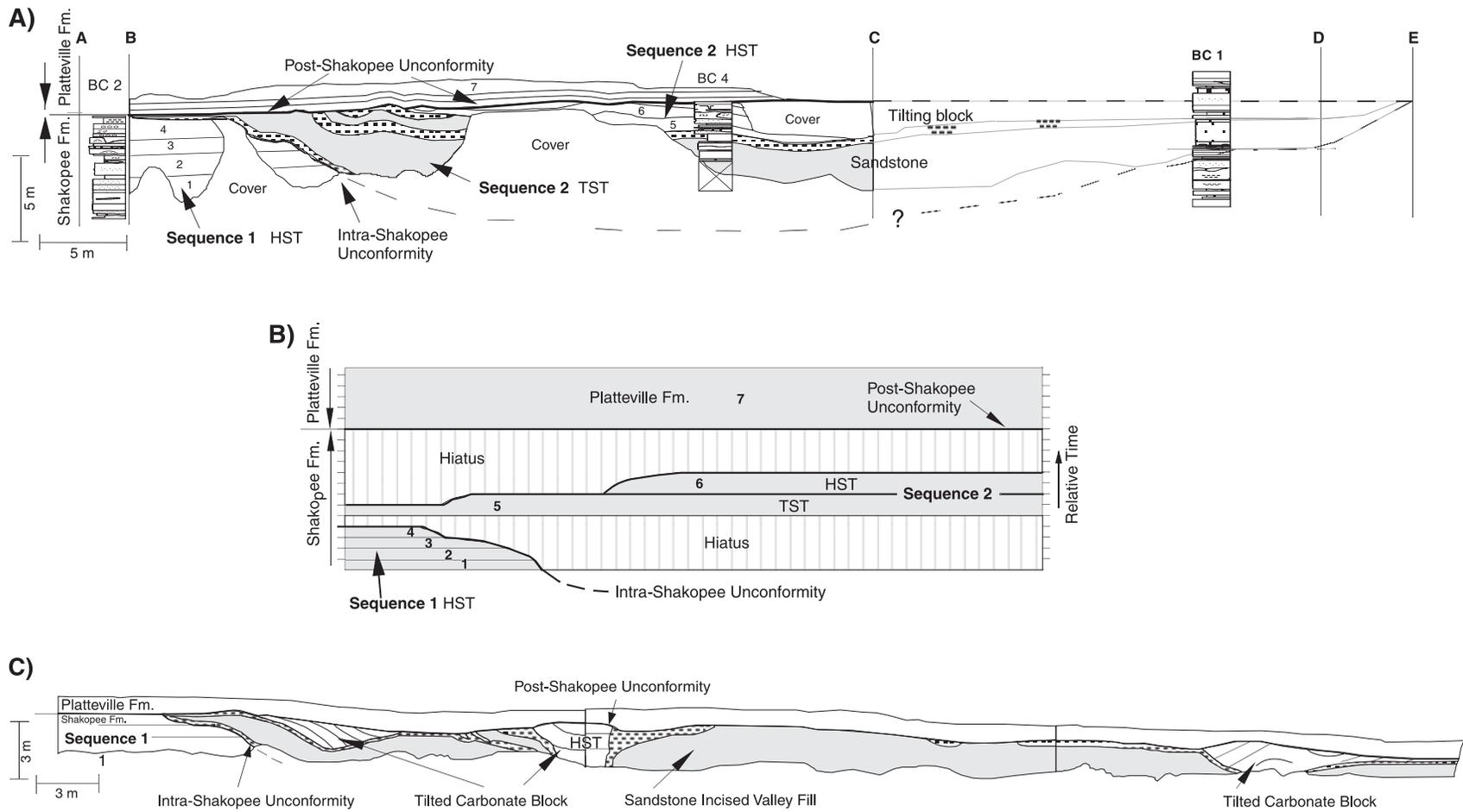
**Figure 4.** Cross sections and Wheeler diagram from Michaels Quarry–Ben Carrie. **A.** Cross section with stratigraphic sections illustrating the west axis of the incised valley system. **B.** Wheeler diagram illustrating depositional sequences 1 and 2, hiatus periods of no deposition, and the two unconformities. **C.** Cross section illustrating east axis of the incised valley, tilted carbonate blocks, and convoluted shale beds.
