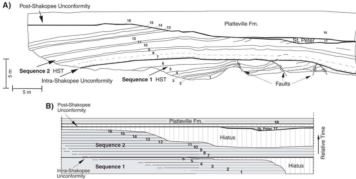
**Figure 3.** Cross section and Wheeler diagram from Ripon Lime and Materials Quarry. **A.** Cross section illustrating the unconformities, strata, truncation, congruent and incongruent tilting, and normal faulting. **B.** Wheeler diagram illustrating depositional sequences 1 and 2, hiatus periods of no deposition, and the two unconformities.
