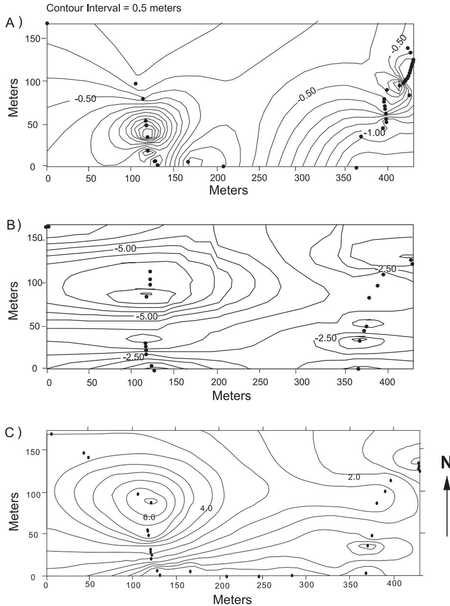
**Figure 5.** Contour and isopach maps created with a total station at Michaels Quarry–Ben Carrie. **A.** Contour map of St. Peter–Platteville unconformity. **B.** Contour map of the intra-Shakopee unconformity, illustrating the east-west axis orientation of the incised valley. **C.** Isopach map of sequence 2, illustrating the shape of the incised valley fill.
