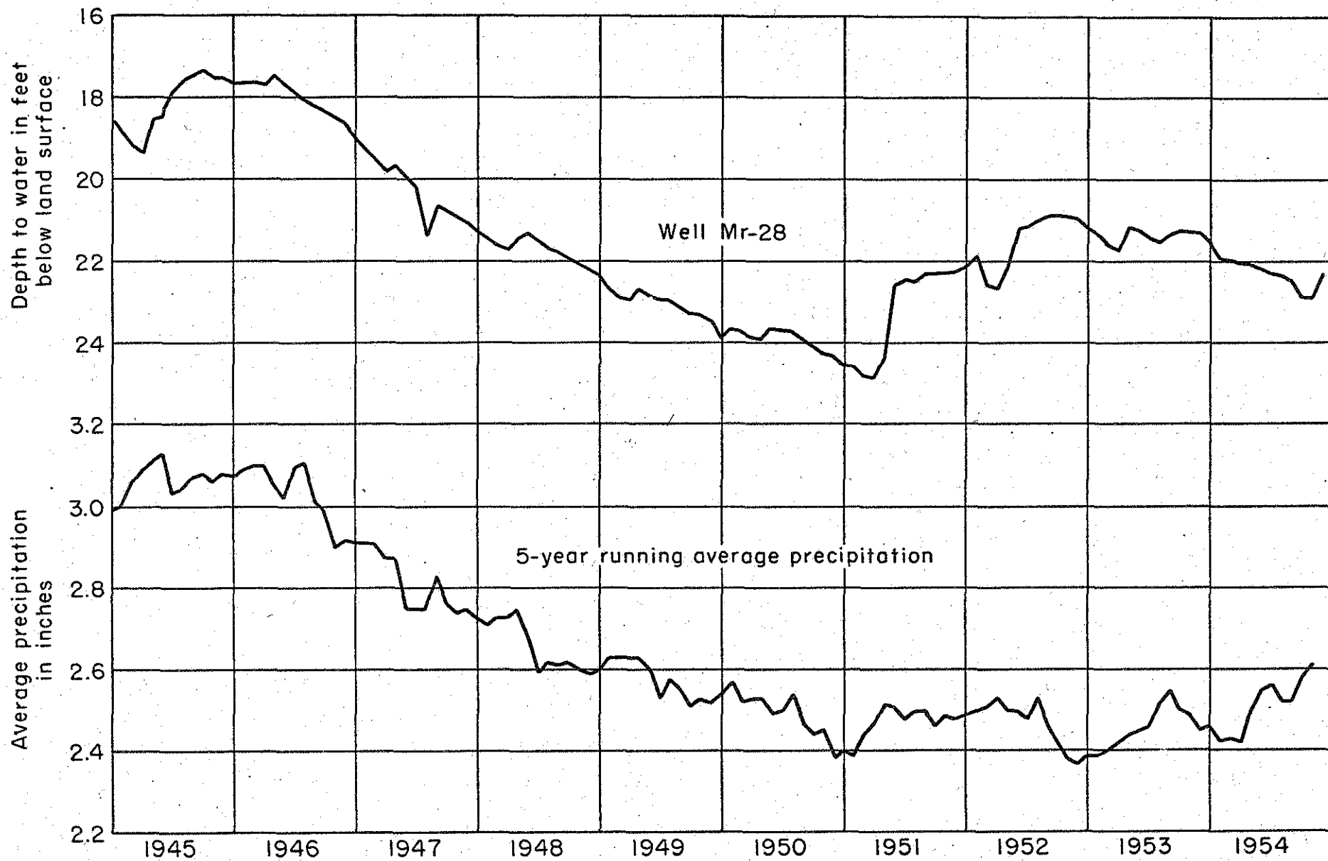
Figure 4.--Water levels in well Mr-28 and 5-year average precipitation at Wausau, Wis., 1945-54.
