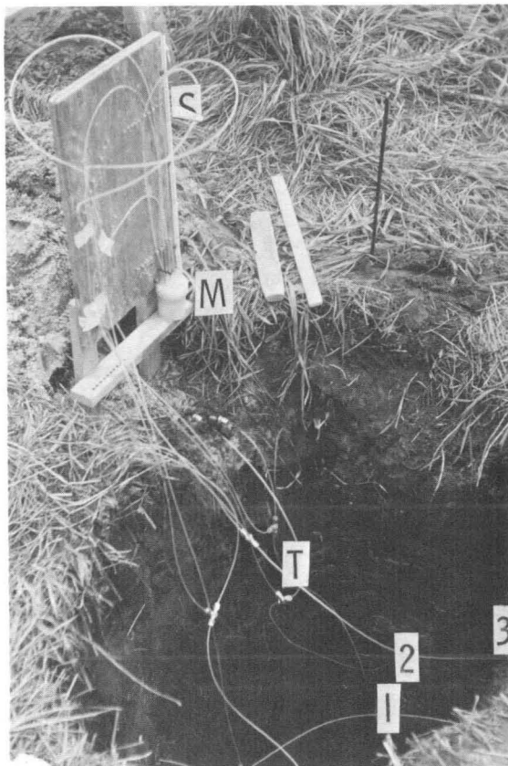
Photo 5.1. Apparatus for field measurement of soil moisture tensions. The 1/8-inch plastic tubes (T) are filled with water and connect pencil-sized tensiometers (inserted into the soil at points 1, 2 and 3) to mercury cup M. Moisture tension in the soil is determined by reading the equilibrium level of the mercury column in the tube along the calibrated scale, S.
