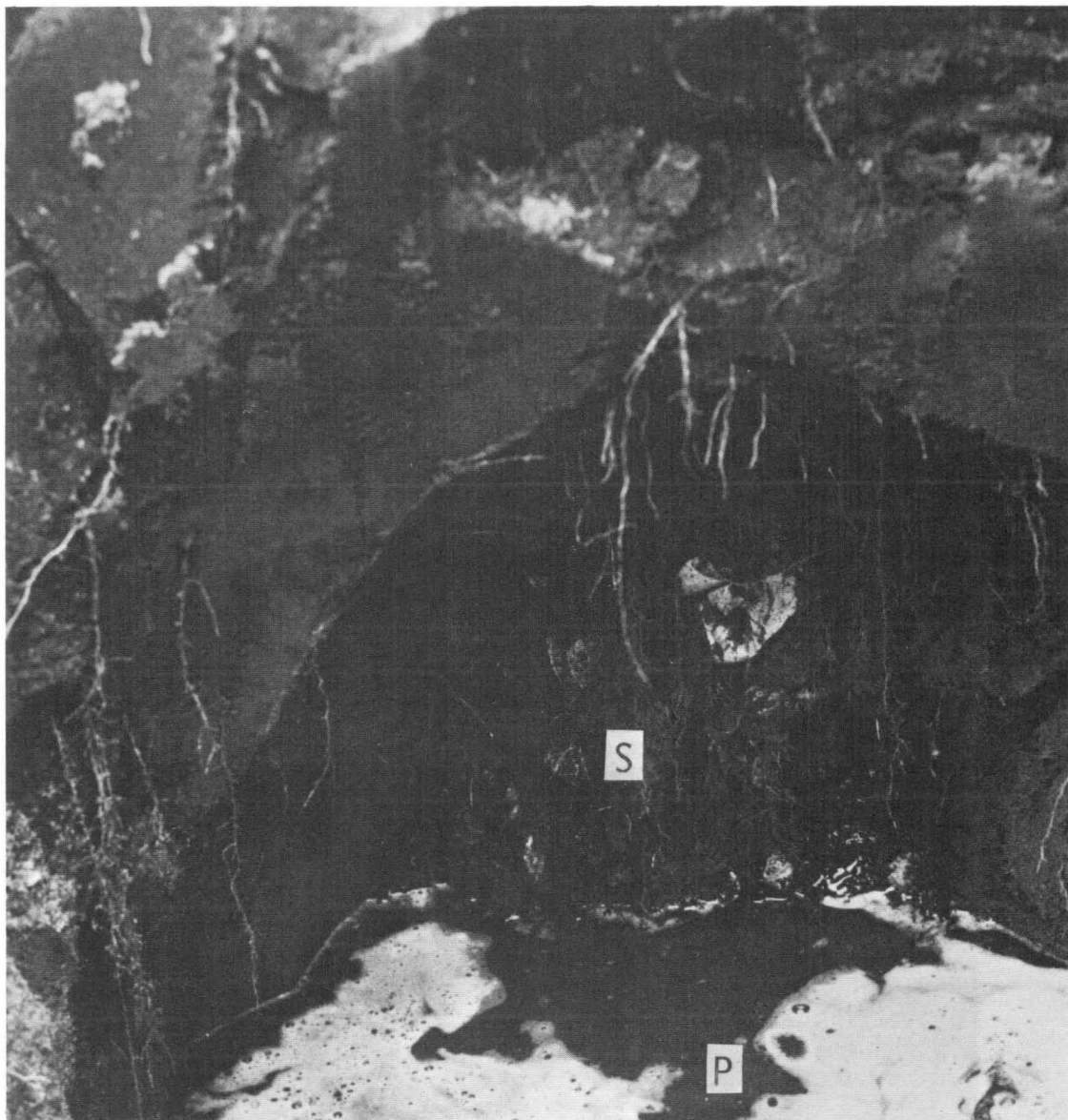
Photo 5.4. Excavated seepage bed (S) (note gravel and abundant root development) of disposal system 1 (Adams County). The sand surrounding the seepage bed had a high K_{sat} of 500 cm/day. However, effluent was ponded in the bed due to crusting which induced a tension of 23 mbar in the surrounding unsaturated soil. The crust was punctured at one time and effluent flowed from the bed into the adjacent pit (P) where it seeped away in minutes through the very permeable uncrusted sand.
