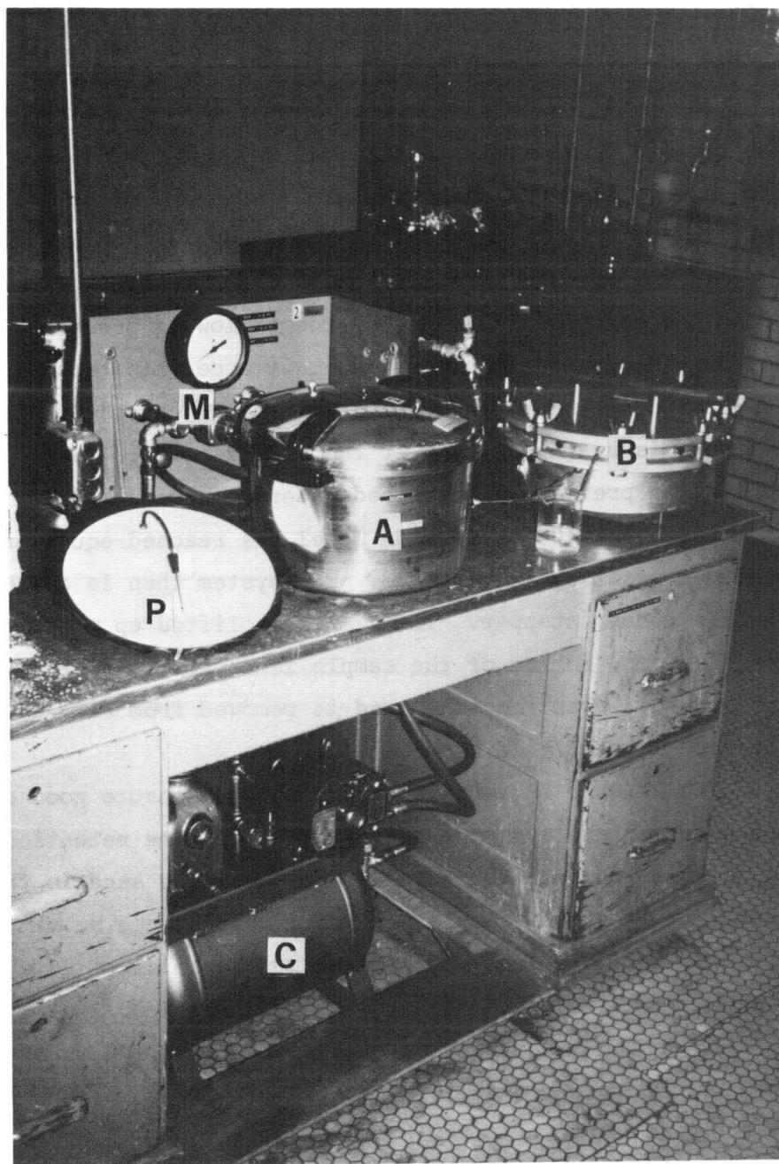
Fig. 3.5. Laboratory setup of a series of pressure extractors for moisture retention measurements between 0.1-15 bar pressure. A = pressure extractor for measurements in the range 0.1-1 bar, B = extractor for measurements up till 15 bar pressure. C = compressor, P = pressure plate cell, M = manifold for pressure regulating for pressure extractors.
