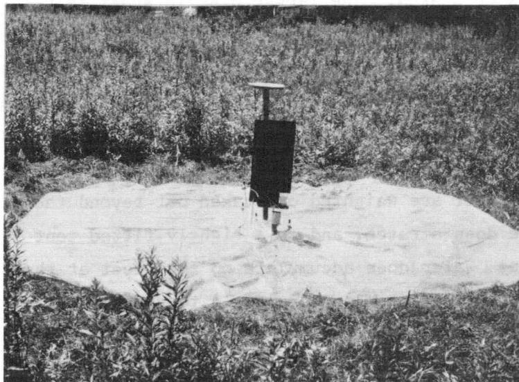
Fig. 3.20. Picture of prepared plot for the instantaneous-profile method with the first plastic sheet in position.
