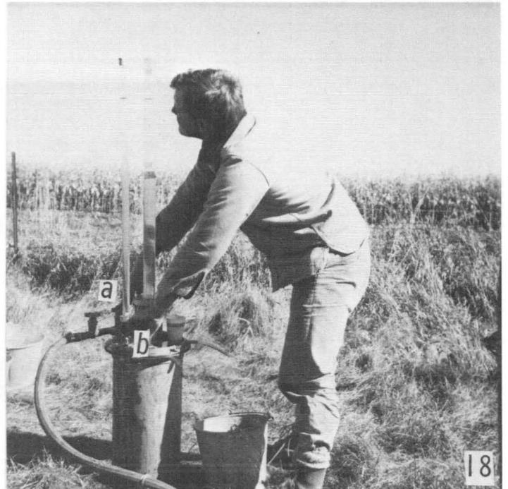
Fig. 3.8. continued. 12 = energy breaker, 13 = outer tube in test hole, 14 = water hose, 15 = reference rod, 16 = assembled inner tube and top plate, 17 = OTS-full measurement, 18 = equal level measurement.
