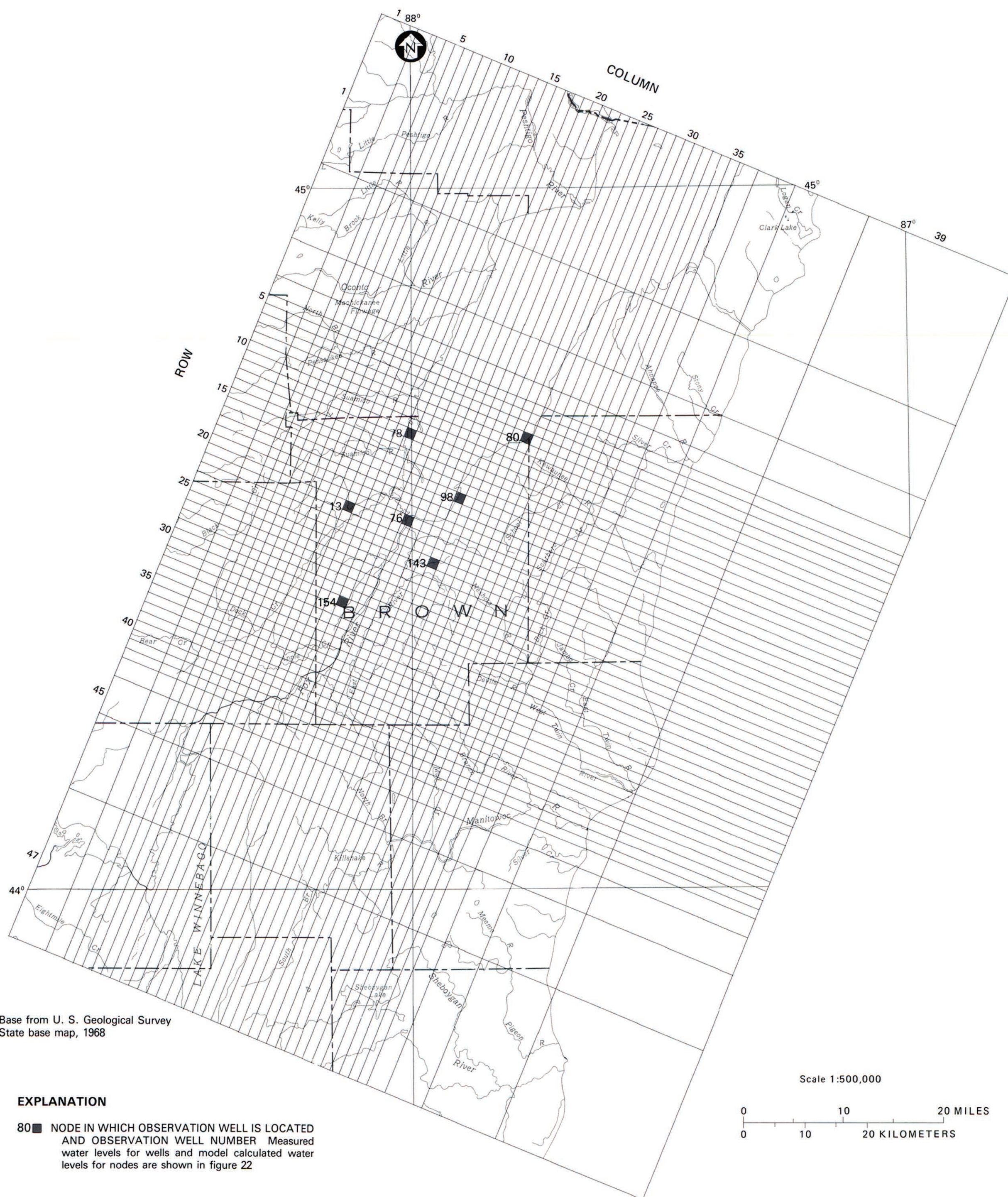
PLATE 2. FINITE-DIFFERENCE GRID AND OBSERVATION WELL LOCATIONS, BROWN COUNTY, WISCONSIN, USED TO CALIBRATE MODEL
