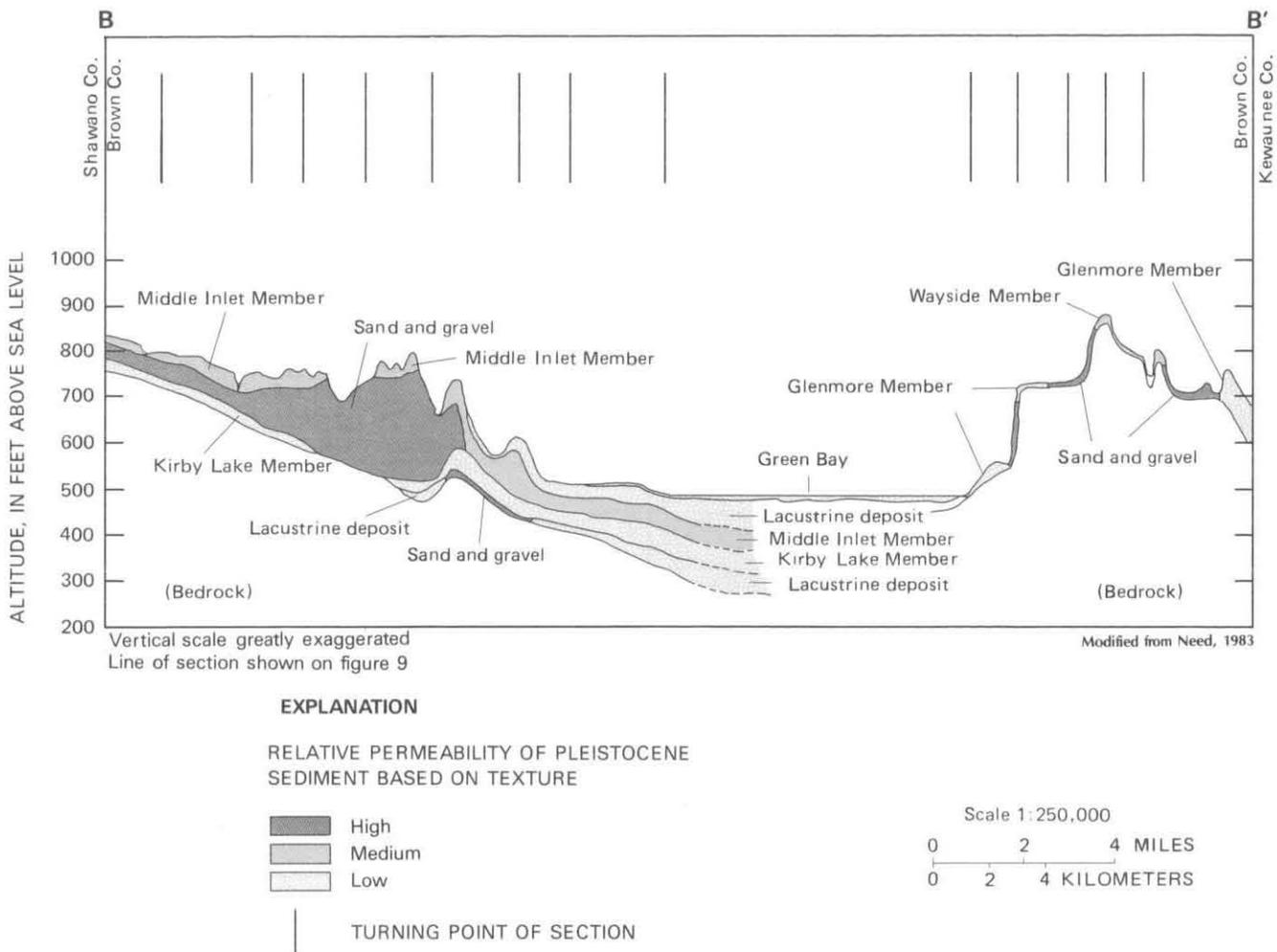
**Figure 6.** Geologic section through and relative permeability of Pleistocene deposits.
