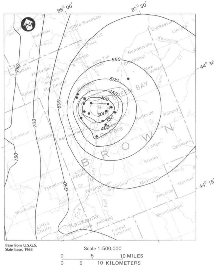
**Figure 20.** Measured and model-calculated potentiometric surfaces in the composite St. Peter and Elk Mound aquifers, 1957.
