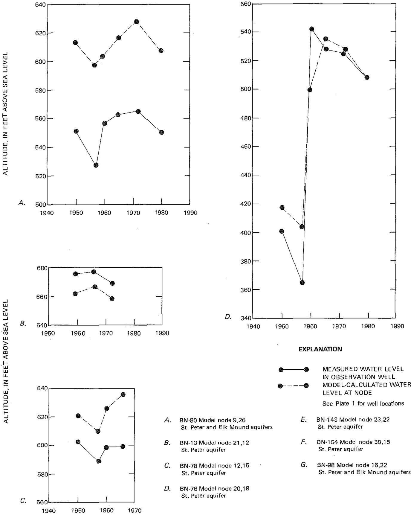
**Figure 22.** Measured and model-calculated hydraulic heads for selected wells in Brown County and corresponding model nodes.
