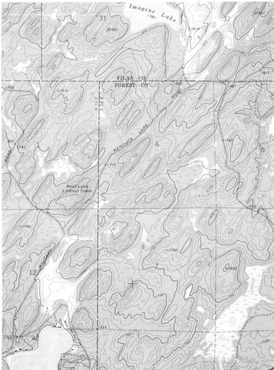
Figure 5 Part of U.S. Geological Survey Anvil Lake Quadrangle, 7.5-minute series, topographic, showing typical drumlins of the county (T. 40 N., R. 12 E.).
