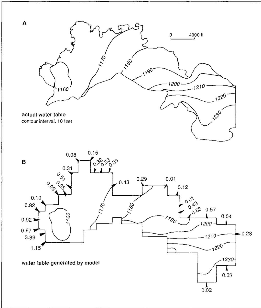
**Figure 19.** Comparison between actual water table (A) and water table generated by calibrated model (B). Contour interval 10 ft. Arrows on (B) indicate flow direction, either to or from specified head nodes. Corresponding numbers indicate magnitude of flow in cubic ft per second.
