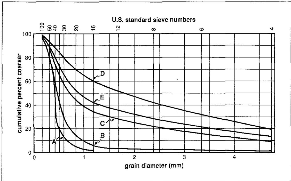
**Figure 8.** Graphs of grain-size analyses for five samples from the same borehole in the Wausau aquifer. The depths from which samples are recovered are 100 to 115 ft (A), 115 to 125 ft (B), 125 to 130 ft (C), 130 to 135 ft (D), and 135 to 150 ft (E). Source: Sand analysis report to city of Wausau for test well at Bugbee and Tienery Streets.
