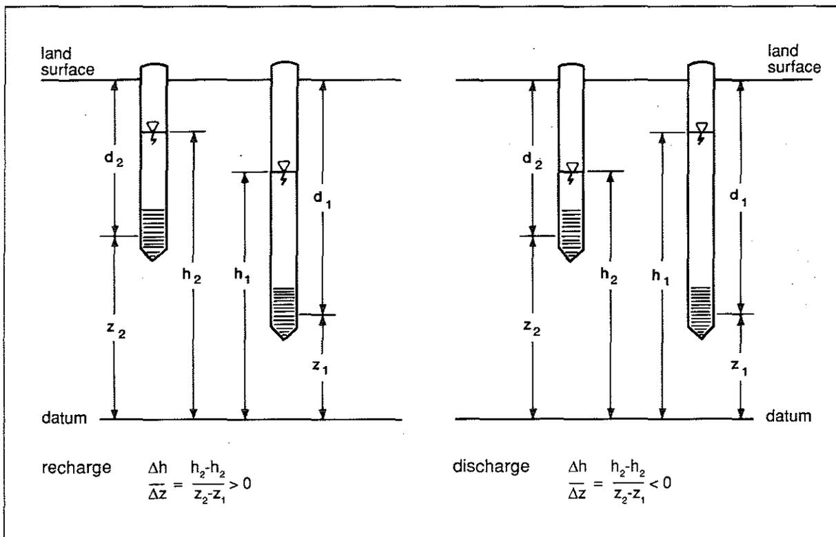
**Figure 16.** Piezometer nest for determining vertical hydraulic gradient. The gradient is positive and flow is directed downward in recharge areas; the gradient is negative and flow is directed upward in discharge areas.
