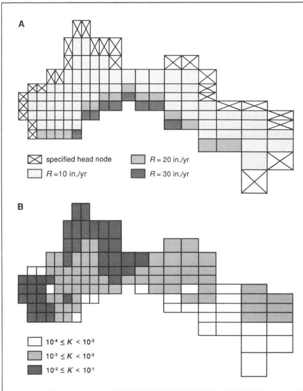
Figure 18. A. Areal distribution of recharge assigned to calibrated model. B. Areal distribution of hydraulic conductivity assigned to calibrated model.
