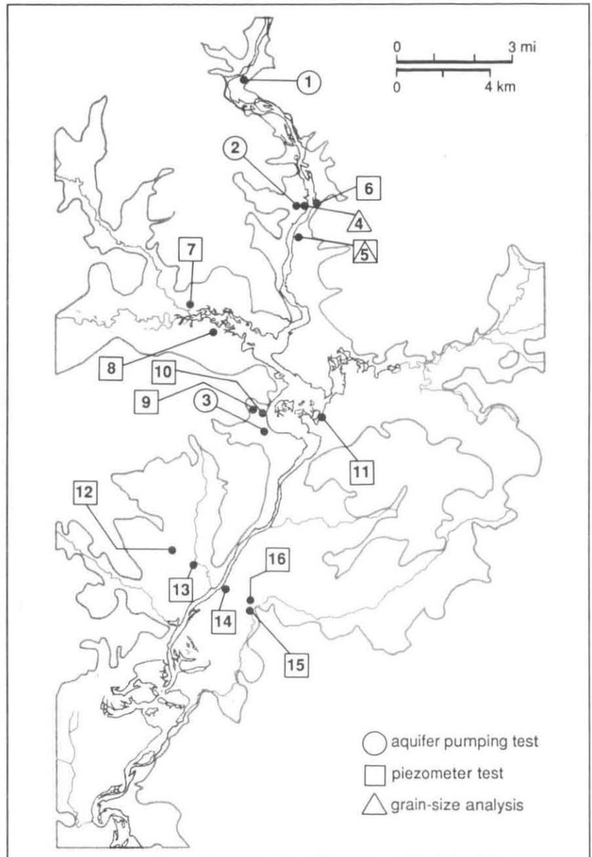
**Figure 14.** Locations of aquifer pumping tests, piezometer tests, and samples for grain-size analyses discussed in text.
