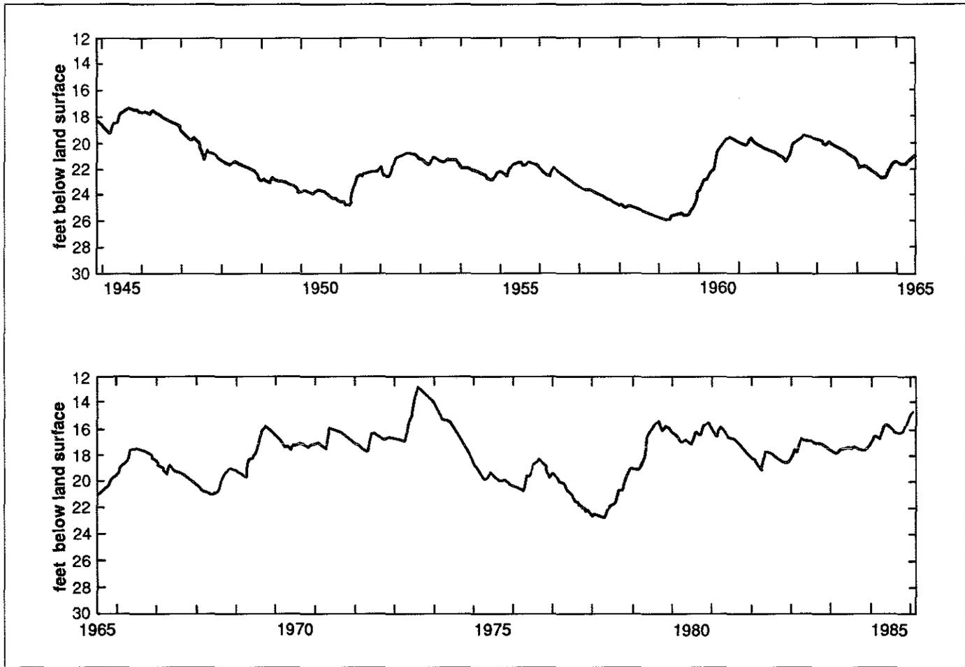
Figure 13. Hydrograph of well MR-28, 1945-85, used to standardize all other reported groundwater levels for plate 2. For location see figure A-1, site 6.
