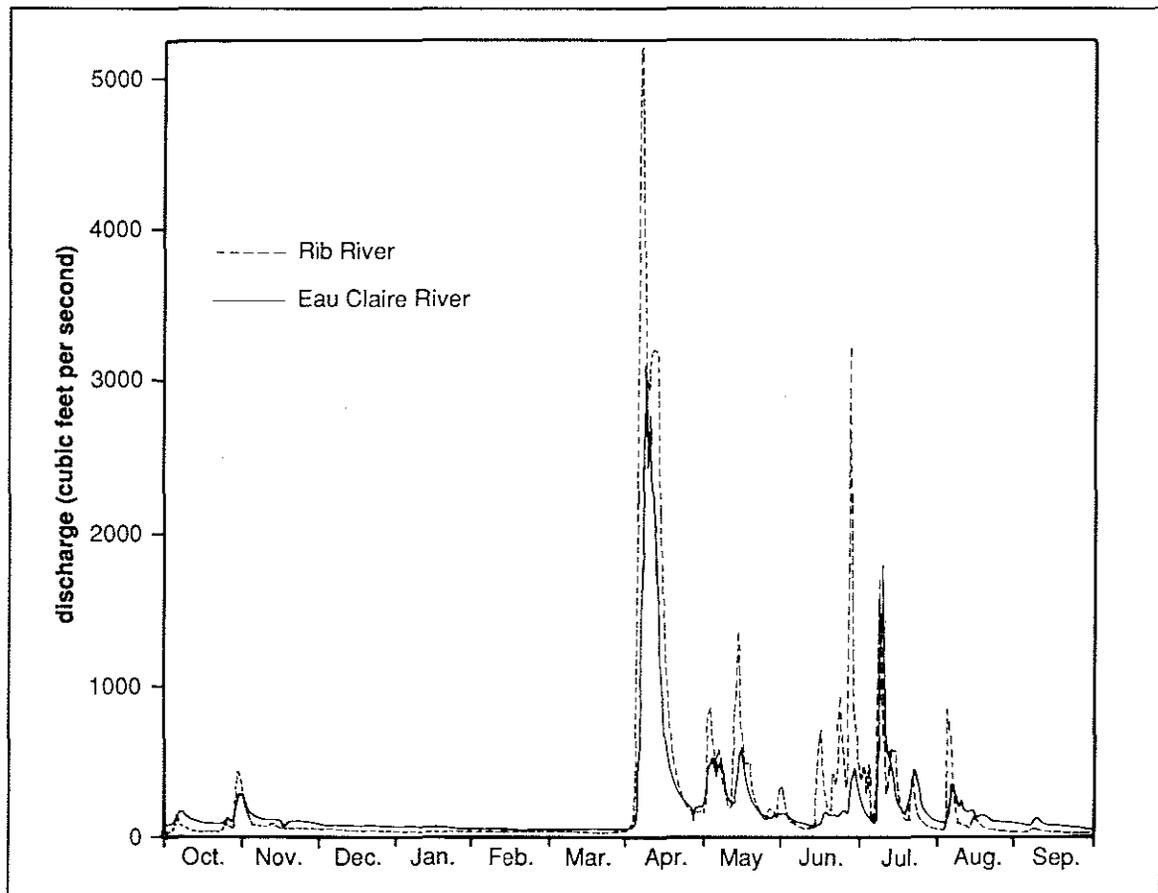
**Figure 12.** Hydrographs of Rib and Eau Claire Rivers in Marathon County, 1955-56. The Rib River has "flashy" discharge because its relatively impermeable, clayey valley promotes overland flow; the permeable sand in the Eau Claire River valley allows more precipitation to infiltrate to the aquifer. As groundwater, it then provides a steady base flow into the Eau Claire River.
