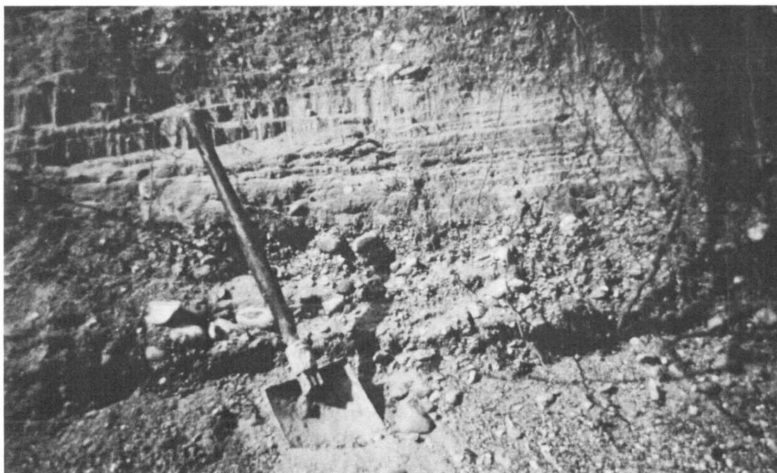
**Figure 6.** Outcrop of material similar to that making up the Wausau aquifer, illustrating heterogeneity of the deposits. Note large variety of grain sizes present.
