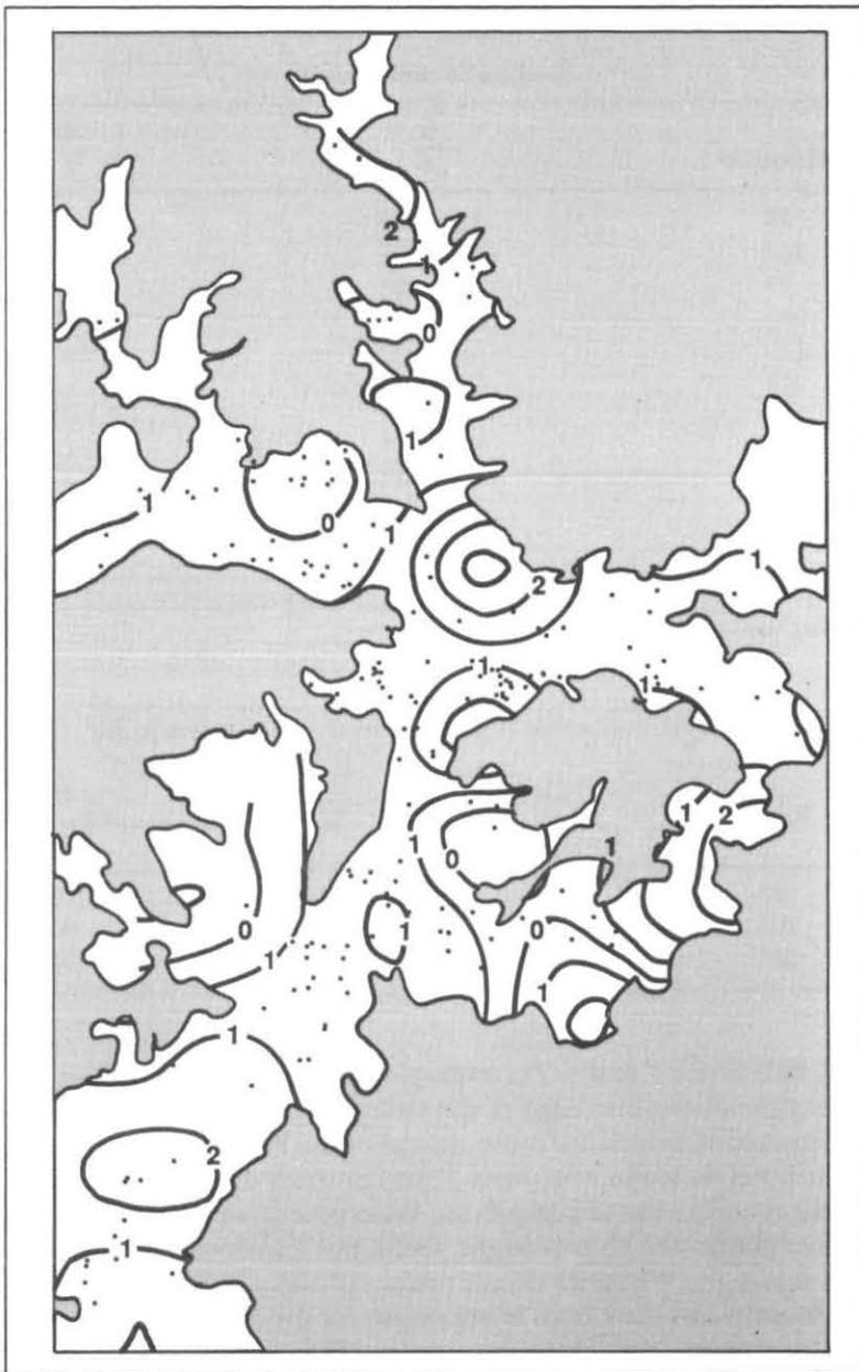
**Figure 15.** Contour map of specific capacity of the Wausau aquifer. Dots indicate data points. Contours represent logarithms (base 10) of specific capacity in gallons per minute per foot of drawdown. For example, the contour line labeled "1" corresponds to a specific capacity of 10 gpm/ft, and the contour labeled "2" corresponds to 100 gpm/ft. Areas of high specific capacity produce high yields to wells. Contour interval is one log<sub>10</sub> unit.
