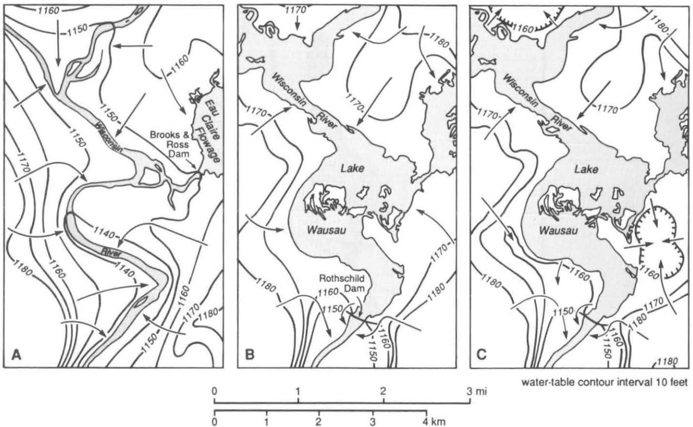
**Figure 3.** Probable effects of dam construction and well pumping on groundwater flow regime near Rothschild. Arrows indicate general groundwater flow directions.
