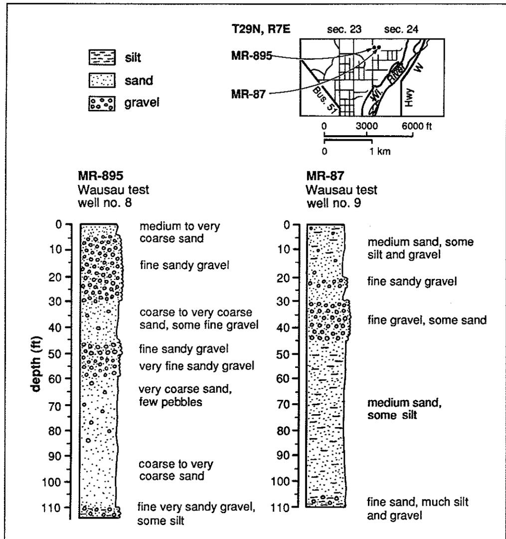
**Figure 10.** Stratigraphy of two sites in north Wausau. Sand and gravel beds are difficult to correlate because of the heterogeneous nature of braided outwash deposits. The two sites are less than 500 ft apart.
