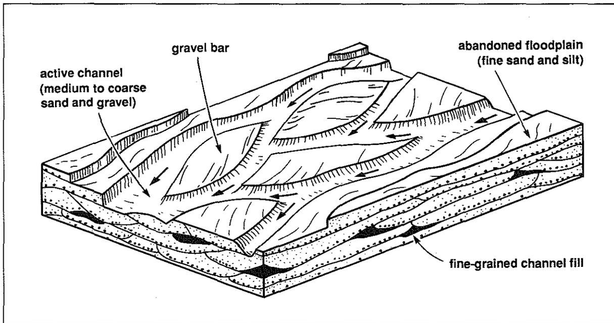
**Figure 9.** *Surficial and subsurface features of braided stream deposits. Lateral channel migration during vertical aggradation results in heterogeneous deposits on all scales. Stratification caused by changing velocities during channel migration results in directional anisotropy. (After Freeze and Cherry, 1979.)*
