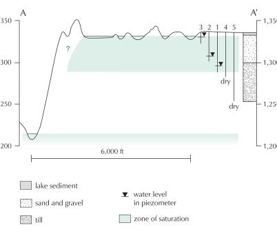
Figure 3. Cross section showing hydrogeology of the Waterman Lake area (modified from Muldoon and others, 1990).
