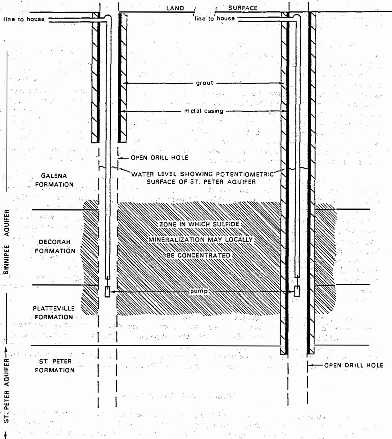
FIGURE 6.— Schematic illustration of the role of well construction in determining if groundwater that has been in contact with oxidized sulfide minerals (sulfates) will enter the well. Well on the left is open to water contaminated with sulfate; the well on the right is not. Movement of sulfate-laden groundwater down into the St. Peter Formation following a head reversal may permit contaminated water to affect newly constructed wells (right).
