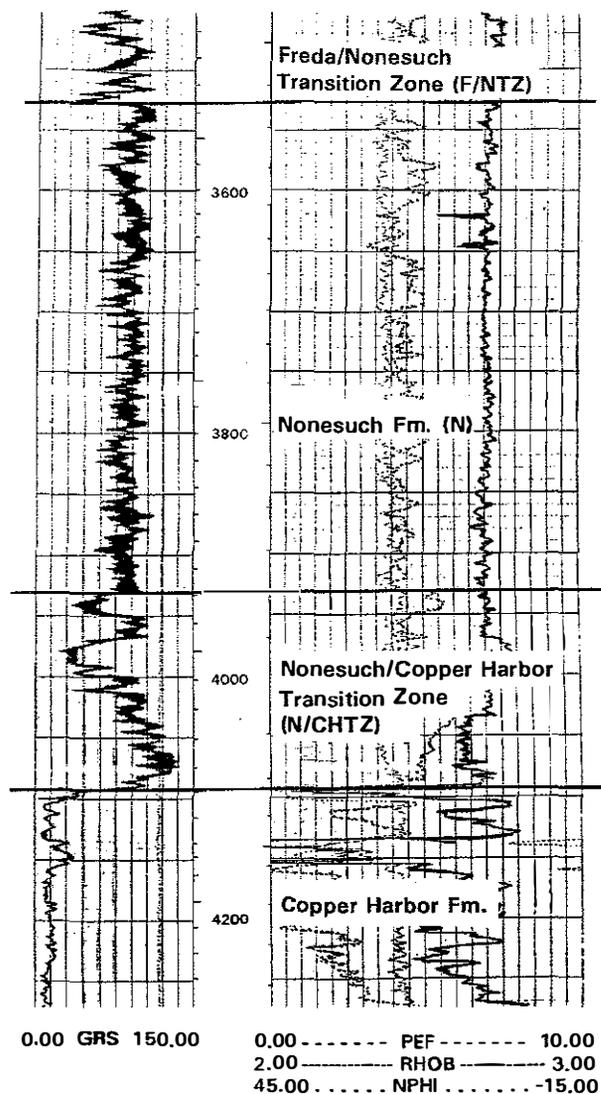
**Figure 1.** Log character of the upper Copper Harbor Formation, Nonesuch-Copper Harbor Transition Zone, and Nonesuch Formation, Terra-Patrick #7-22 borehole, Bayfield Co., Wisconsin. GRS = Spectral Gamma Ray (API); NPHI = neutron porosity (%); PEF = photoelectric factor; RHOB = density (gm/cc).
