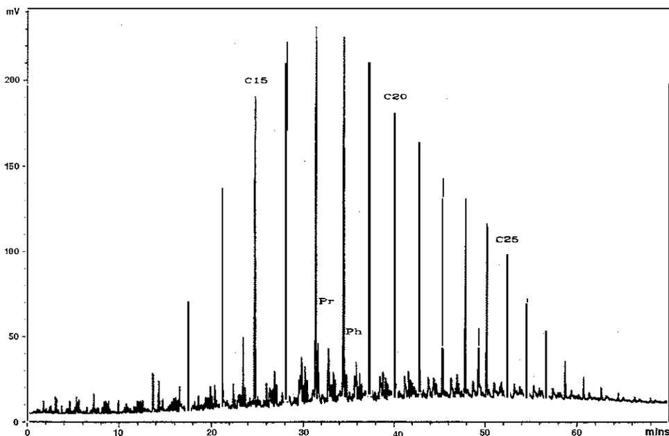
Figure 3. Whole oil gas chromatographic fingerprint of White Pine Copper Mine oil seep.
