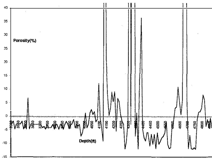
**Figure 2.** *Nonesuch and Copper Harbor Formations. Plot of density porosity (%) vs. depth (feet). A matrix density of 2.65 g/cc was used in calculating porosity values, This matrix density is commonly used for a sandstone lithology. The anomalous spiking below 4,000 ft is due to extreme borehole rugosity.*
