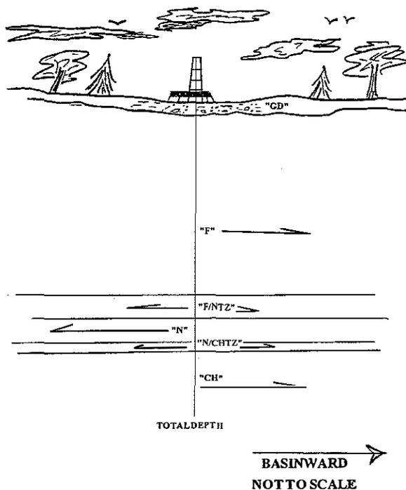
**Figure 3.** Schematic stratigraphic model illustrating the sedimentary sequences penetrated by the Terra-Patrick #7-22 borehole, Bayfield County, Wisconsin. Arrows indicate relative direction of stream flow and/or lacustrine regression/progradation, as appropriate. GD: Glacial drift; F = Freda Formation; F/NTZ = Freda-Nonesuch Transition Zone; N = Nonesuch Formation; N/CHTZ = Nonesuch-Copper Harbor Transition Zone; and CH = Copper Harbor Formation. Not to scale.
