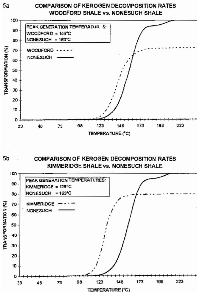
Figure 5. Comparison of transformation rates of (A) Woodford and (B) Kimmeridge kerogens to the Nonesuch Formation based on the Bear Creek WC-26 sample kinetics. The Woodford and Kimmeridge kerogens have been 27 percent and 30 percent transformed to give comparable  $T_{max}$  values as the Nonesuch Formation to offset any difference due to thermal maturity.
