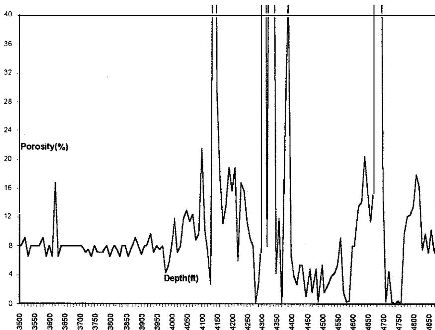
**Figure 1.** *Nonesuch and Copper Harbor Formations. Plot of density porosity (%) vs. depth (feet). A matrix density of 2.85 g/cc is used in calculating porosity values. Cross plots of various log signatures were made in determining this matrix density, The anomalous spiking below 4,000 ft is due to extreme borehole rugosity.*
