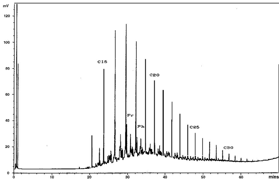
Figure 2. Saturate fraction gas chromatographic fingerprint of Bear Creek WC-26 core hole, Nonesuch Formation.
