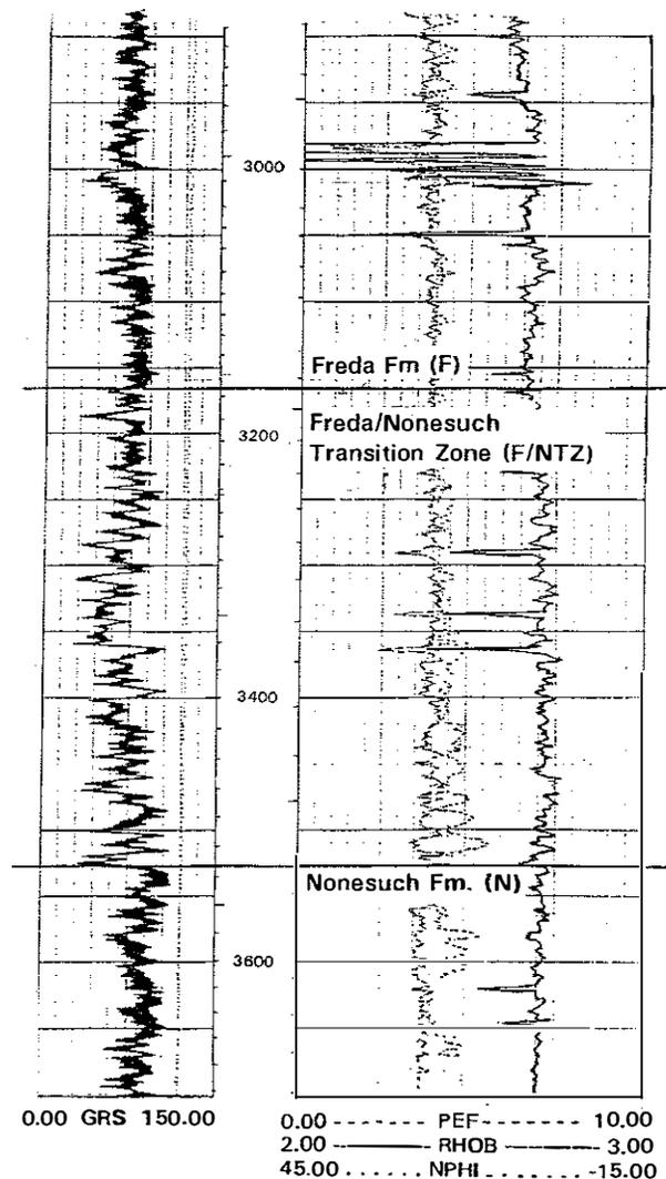
**Figure 2.** Log character of the Freda-Nonesuch Transition Zone and lower Freda Formation, Terra-Patrick #7-22 borehole, Bayfield Co., Wisconsin. GRS = Spectral Gamma Ray (API); NPHI = neutron porosity (%); PEF = photoelectric factor; RHOB = density (gm/cc).
