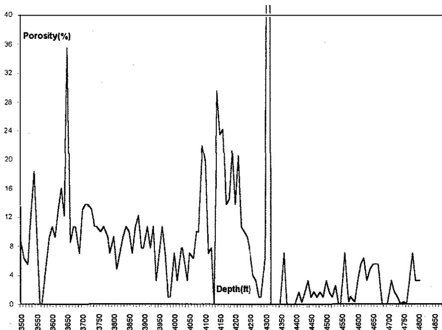
**Figure 3.** *Nonesuch and Copper Harbor Formations. Plot of sonic porosity (%) vs. depth (feet). A matrix travel time of 55.6 sec/ft is used in calculating porosity values. This matrix travel time is commonly used for a sandstone lithology. The anomalous spiking below 4,000 ft is due to extreme borehole rugosity.*
