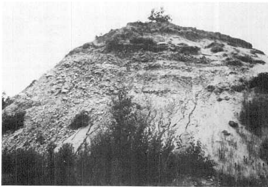
Figure 7. Excavation face at Hamilton Mound quarry showing quartzite blocks in Cambrian sandstone overlying quartzite. Sandstone beds become more regular and flaggy to the right of the photo. Quartzite bluff is to left. Horizontal dimension is about 33 ft (10 m).
