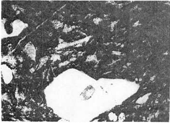
Undeformed shard fragments (white) with quartz phenocryst in rhyolite tuff from Utley. x25.
