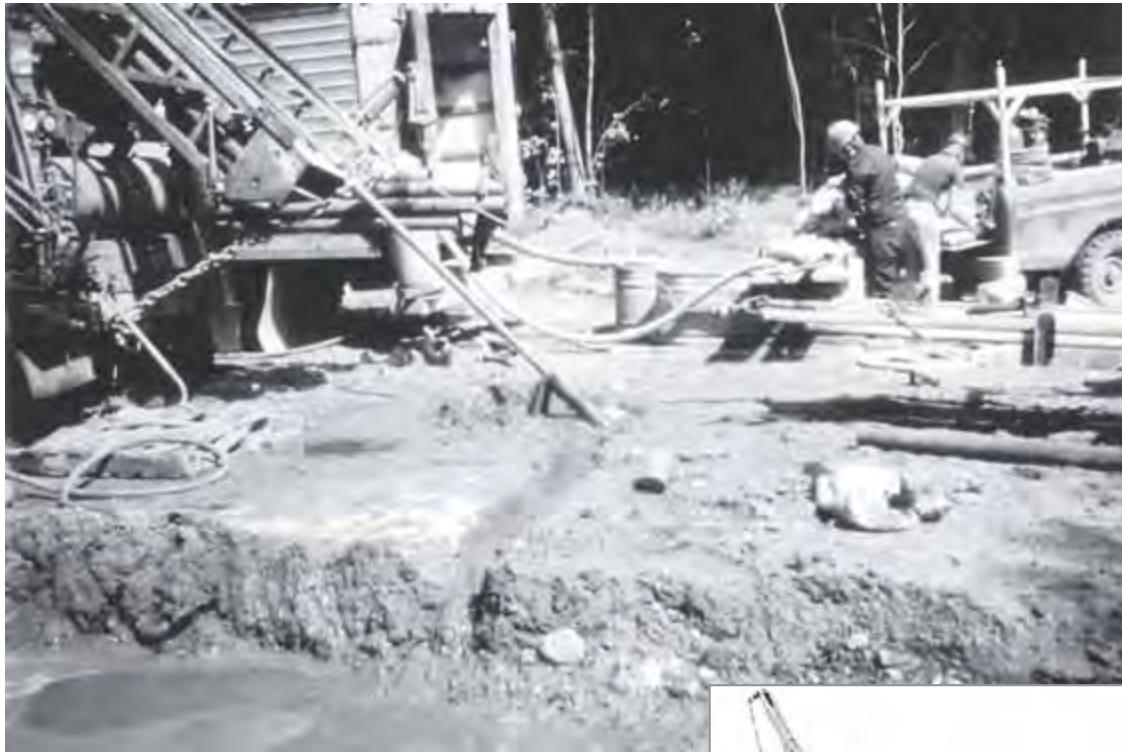
Exploration (drilling) for metallic mineral occurrences in northern Wisconsin is shown in photograph above. About 0.25 acre of land is affected by each drillhole constructed. The drilling mast is placed at an angle to intersect the typically inclined rock strata as nearly perpendicular as feasible (see drawing, right).
