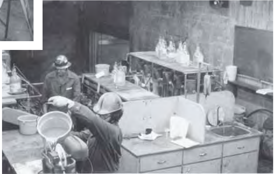
A bulk sample of potential ore material (above) may be collected for testing and evaluation in special laboratories that simulate mineral-processing facilities or mills, such as the laboratory (right) of the Lakefield Research Center in Ontario, Canada.
