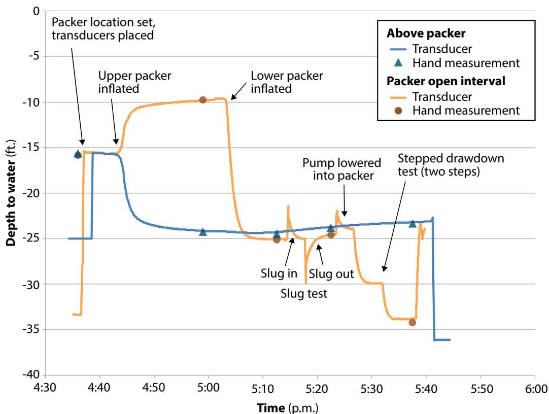
**Figure 12.** Straddle packer data for testing at 170 feet.
