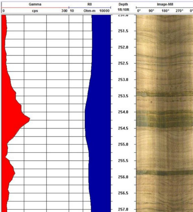
**Figure 5.** Gamma, normal resistivity, and optical log from 251 to 257 feet.
