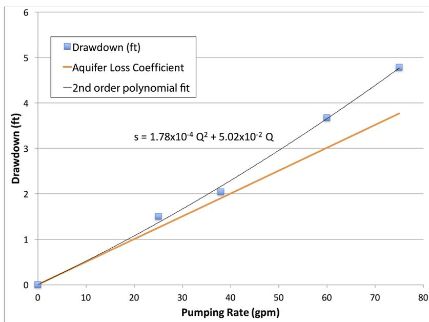
Figure 10. Stepped drawdown test.
