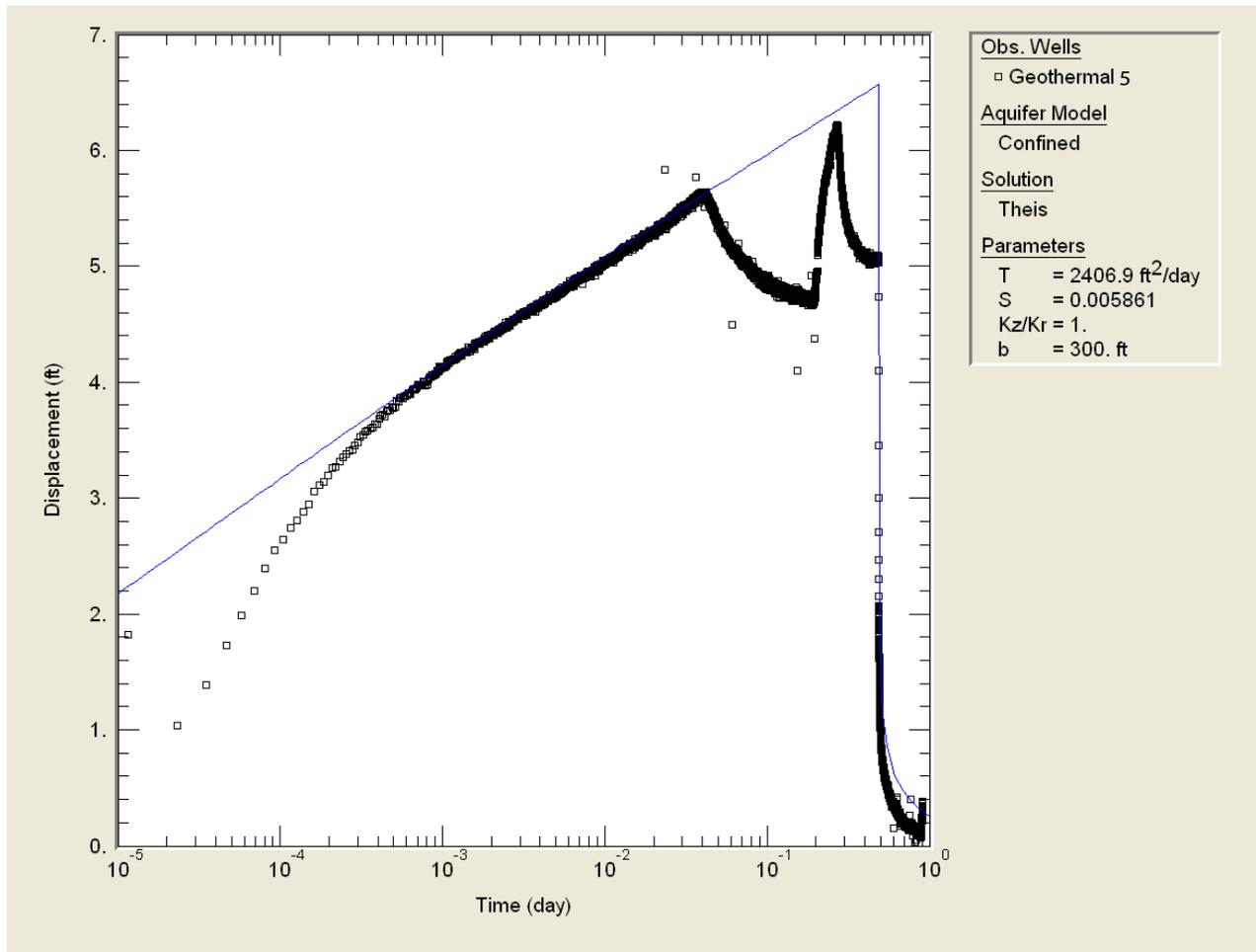
**Figure 8.** Results of 12-hour pumping test using Aqtesolv® and the Theis equation.
