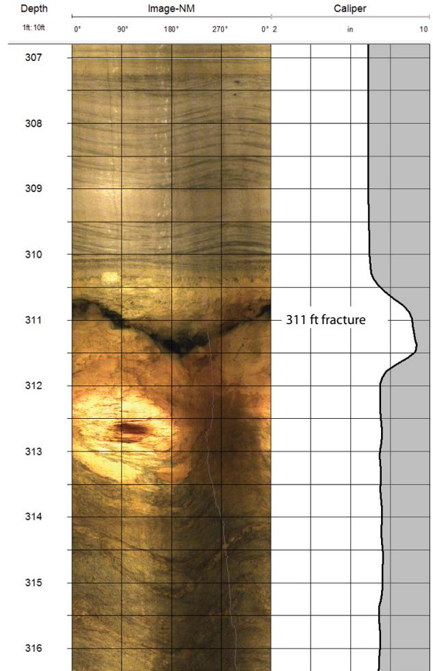
**Figure 6b.** Fracture at the contact between the sandstone and the crystalline rock at 311 feet.
