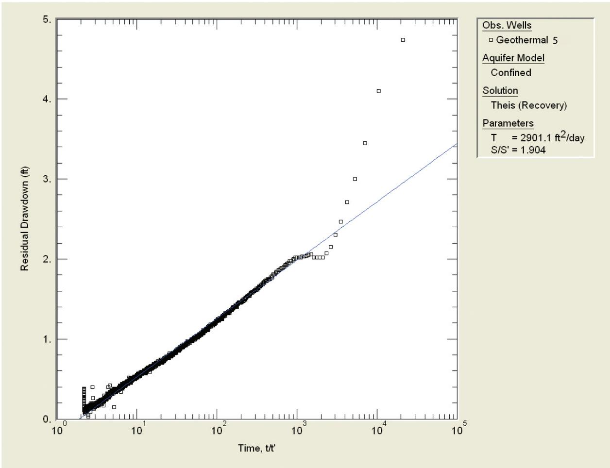
**Figure 9.** Results of 12-hour recovery test data using Aqtesolv® and the Theis recovery equation.
