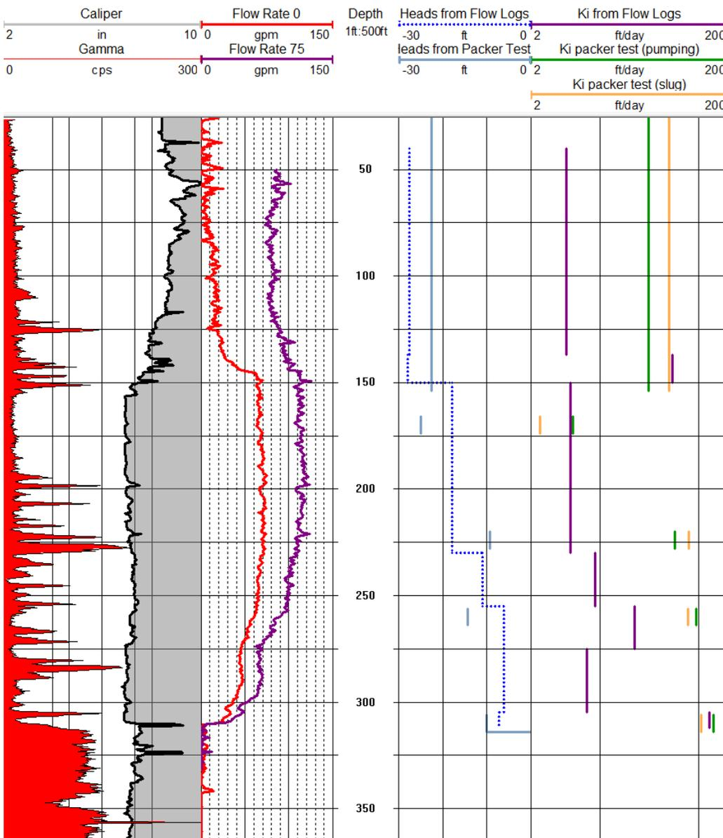
Figure 11. Flow logging and packer testing results. Flow is upward.
