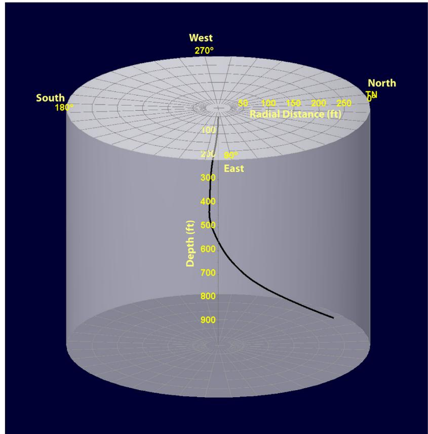
Figure 4. Deviation log of Geothermal Test Well 5.
