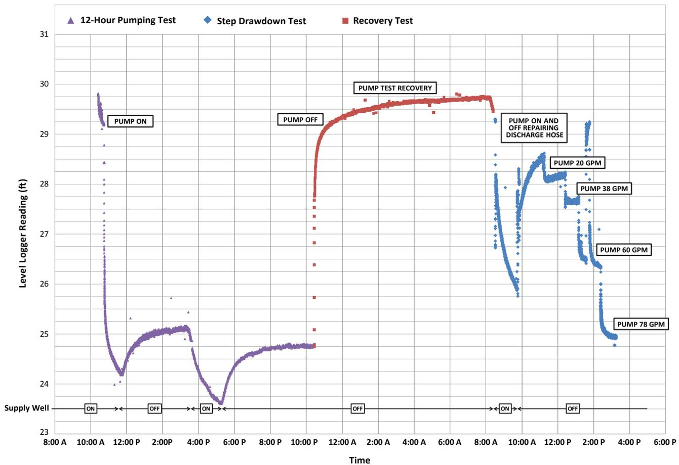
**Figure 7.** Water level data from 12-hour pumping test and recovery, and the 8-hour, stepped drawdown test. Periods when the data was affected by a supply well are shown above.
