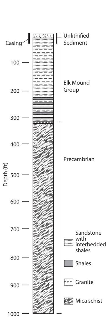
**Figure 2.** Lithology of Geothermal Test Well 5.
