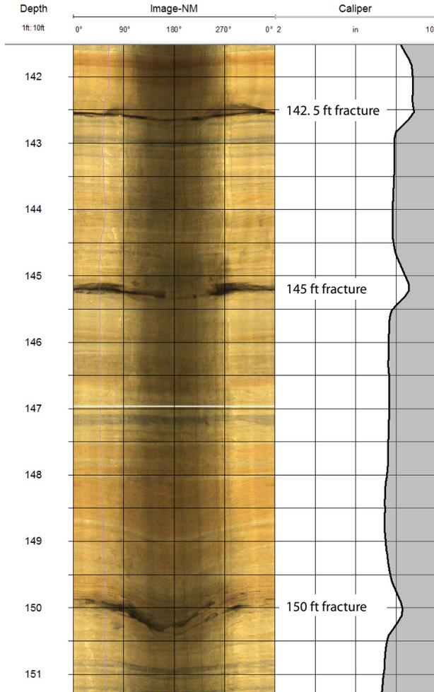
**Figure 6a.** Three fractures in the well at 142.5, 145, and 150 feet depth.
