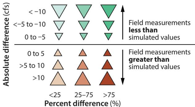
Residuals are calculated as measured value minus simulated value. **Symbol size** indicates absolute difference; **symbol shading** indicates percent difference between simulated and measured values.
