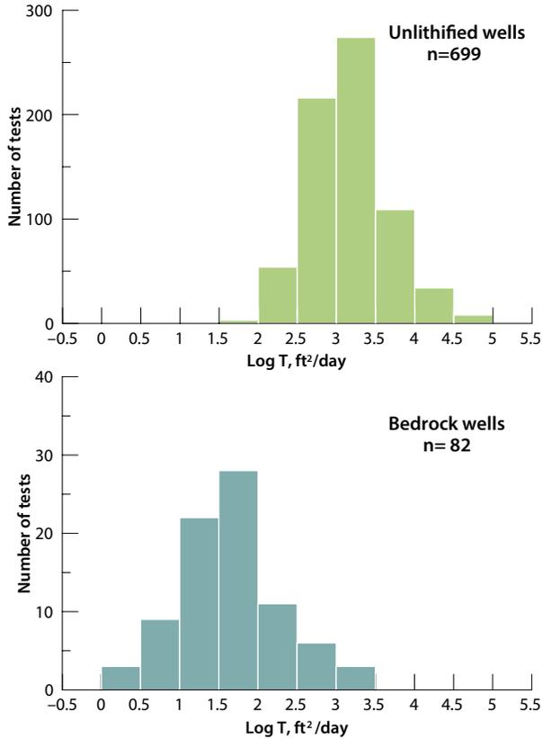
**Figure 3c.** Specific-capacity test results in the Park Falls Unit.
