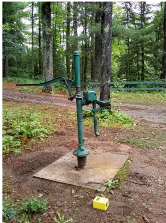
Figure 6. Example of control measurement used for HVSR calibration. The Tromino seismometer is placed directly next to a well where depth to bedrock is indicated by driller's well records.
