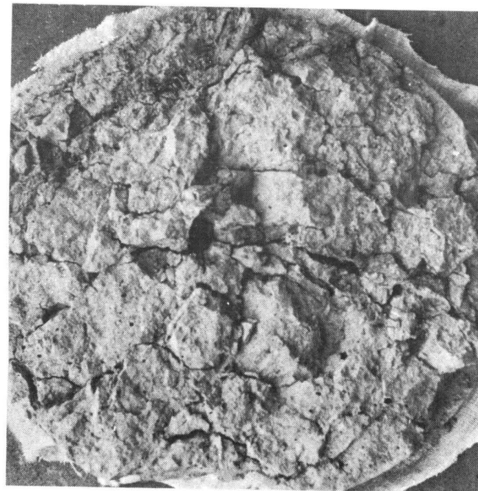
Oshkosh clay (cultivated) B 3 (80cm). Structure: Moderate MEDIUM prismatic breaking into strong medium angular blocky. K: 5 cm/day. B.D.: 1.52 P.V.: 44% Part.dens.: 2.73.
