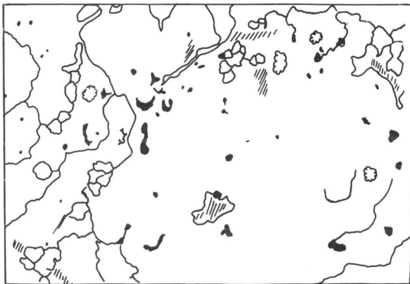
St.Charles-Bavaria silt loam (Charmany farm).Ap (20cm) Structure: apedal with clods. K: 11 cm/day. B.D.: 1.37 P.V.: 46% Part.dens.: 2.55.
