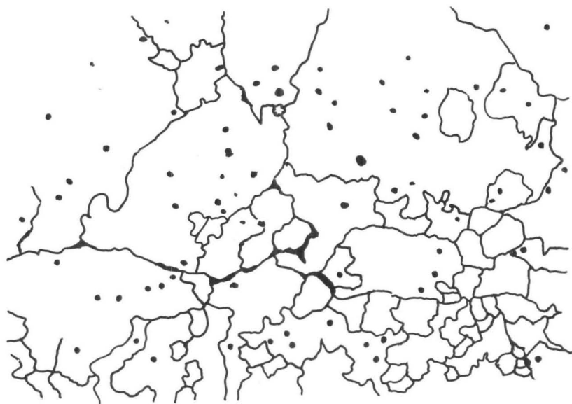
Tama silt loam(cultivated) A2 (20 cm).Structure: Weak medium platy and moderate very fine subangular blocky. K: 11 cm/day B.D: 1.37 P.V: 47% Part.dens: 2.57.
