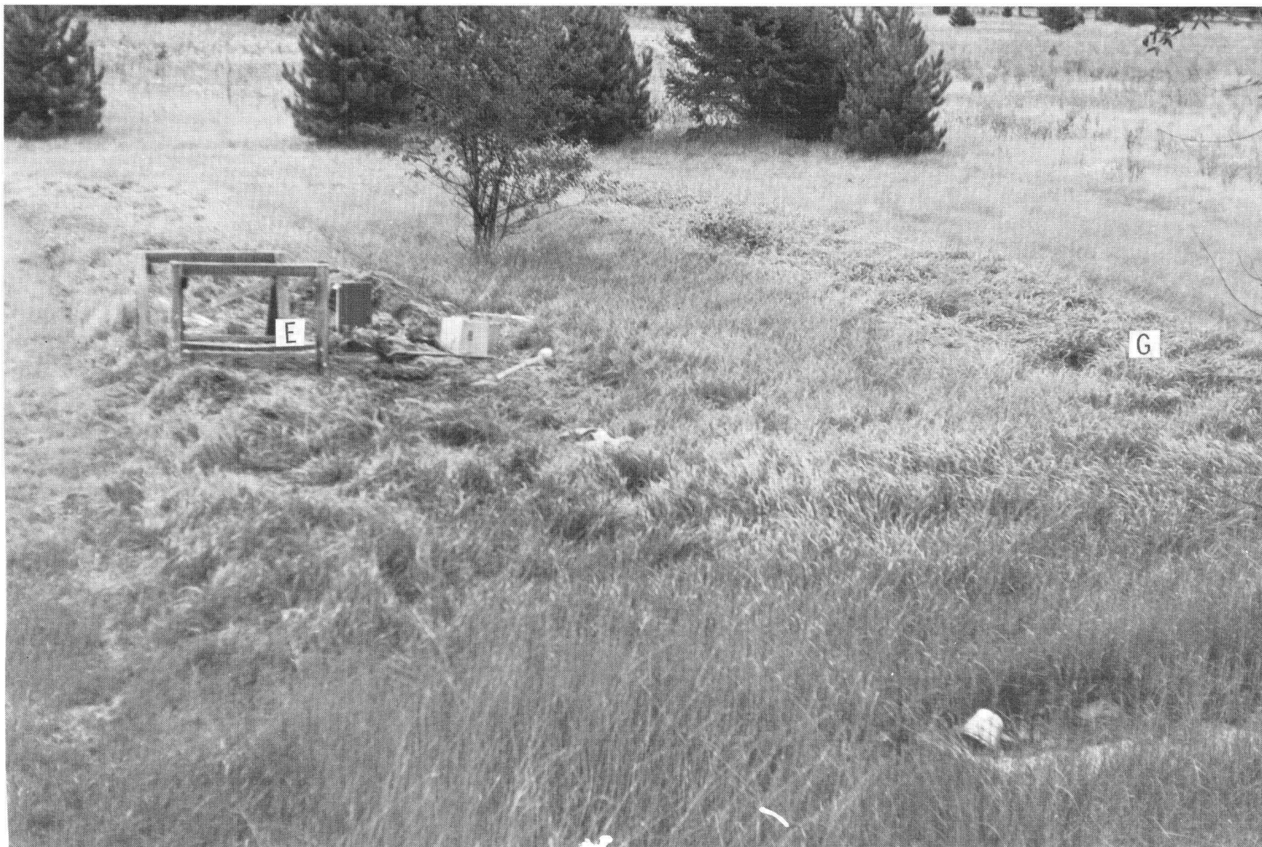
Photo 3.4.2b Absorption field in Plainfield loamy sand at Friendship. The location of the seepage beds, which were filled with effluent, is clearly marked by lush growth of grasses (G). An excavation (E) was made next to the middle bed for purposes of sampling and measurement of soil moisture tensions (see diagram of system, Figure 3.4.2).
