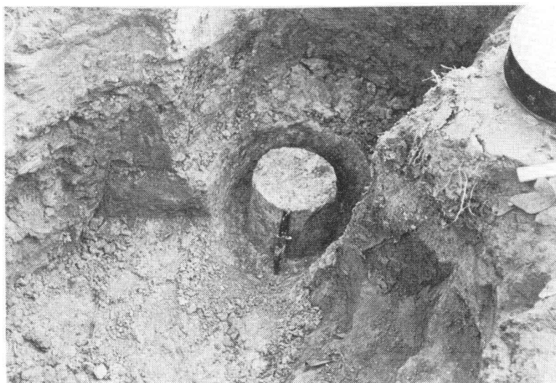
Photo 2.3.3a Cylindrical column of soil, 30 cm high and with a diameter of 25 cm, carved out from the test level downward in situ .
