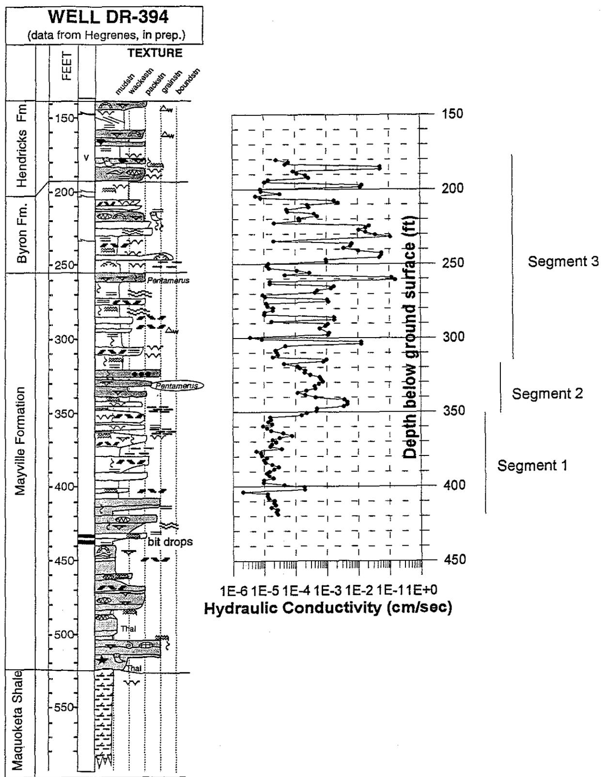
**Figure 3.** Hydraulic conductivity profile for Jarmen Rd. corehole (DR-394, location shown in figure 1) Slug tests were conducted at 1.5-ft intervals using straddle-packers. The profile has been divided into three segments based on variations in hydraulic conductivity. The stratigraphic column, based on descriptions from Hegrenes, (in prep.) is shown to the left of the hydraulic conductivity profile; legend is shown in figure 2.
