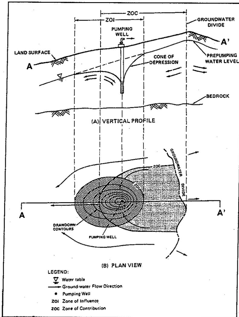
**Figure 2.** Diagram and terminology for wellhead protection in a simple hypothetical groundwater flow system (from USEPA, 1987).
