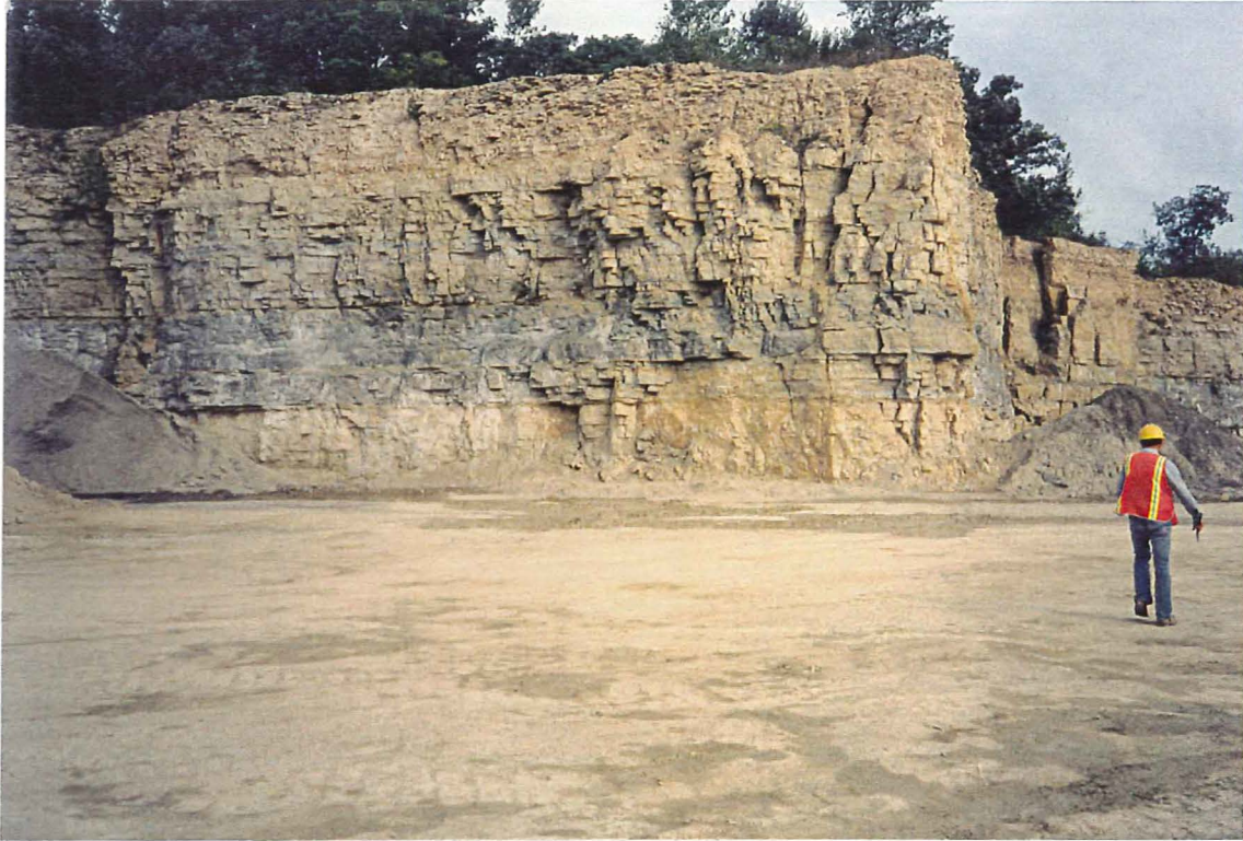
Figure 12. West face of Hausz Brothers quarry (SE-6) Fort Atkinson. Upper third of face is Dunleith Member with pitted weathering. Middle third is Ion plus 3 feet of Decorah. Lower light colored beds are Nachusa Member.
