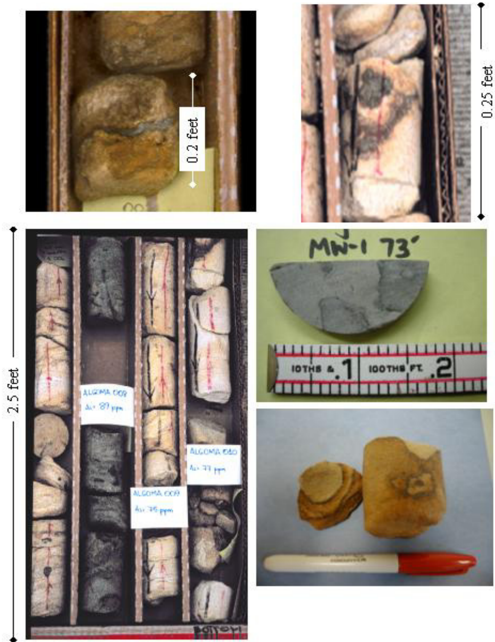
Figure 13b. Photos of core. Upper left: SCH in SB-1. Upper right: nodule and vein with oxidized rim in SB-1. Lower left: SB-1 core, below SCH showing change from oxidized (white to orange) to reduced (gray) sandstone. Mid-right: mineralization in dolomite at 22.3 m (73 feet) below ground surface in MW-1. Lower right: Mineralization with oxidized rim in sandstone.
