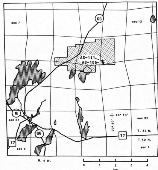
**Figure 2** Map in the vicinity of the Clam Lake anomaly (T. 43 N., R. 4 W., Ashland County, Wisconsin) showing location of bore holes AS-105 and AS-111, and field gravity stations. Area of diagram corresponds to gridding magnetic and gravity modeling; small irregular polygon surrounding bore holes is the outline of the modeled Clam Lake intrusion. Flight lines for the aeromagnetic survey are generally at 800 m spacing along section lines.
