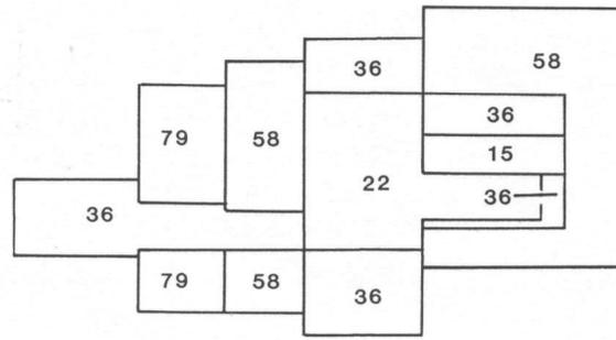
**Figure 9** Plan view of prism model showing depth below surface in meters to the top of the body. See text for discussion.
