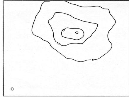
**Figure 8** **a** Observed Bouguer anomaly gravity field. Contour interval, 5 mgal. An additional 10 field stations immediately adjacent to the diagrams were included in the contouring; **b** Residual Bouguer anomaly gravity field. Contour interval, 5 mgal. See text for discussion; **c** Gravity field calculated from model. Contour interval, 5 mgal.
