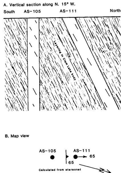
**Figure 4** Diagrammatic section through AS-105 (vertical) and AS-111 (inclined) along N. 15° W. showing orientation of layering in the Clam Lake body.
