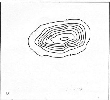
**Figure 7** **a** Observed total intensity magnetic field from J. Karl and Friedel (1975). The survey was flown at an elevation of 150 m above the land surface along north-south flight lines spaced 0.8 km apart. Contour interval, 1000 gammas; **b** Vertical magnetic field after reduction to the present magnetic pole. Contour interval, 1000 gammas; **c** Vertical magnetic field calculated from model. Contour interval, 1000 gammas. See text for discussion
