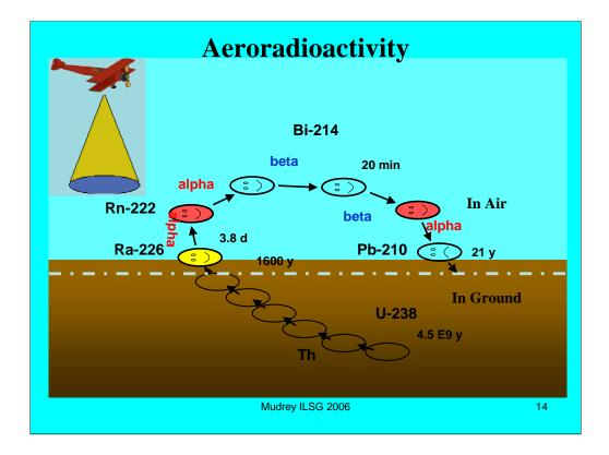
Radon 222 to lead 210 are either gases or aerosols. All of the other nuclides in this greatly simplified diagram are part of the geochemical story. Radium, for instance, behaves as calcium and is concentrated along fractures in dolomite and limestone. Weathering of the carbonate releases the bound radon which then explains the elevated radon found in carbonate terranes and terra rosa soil.
