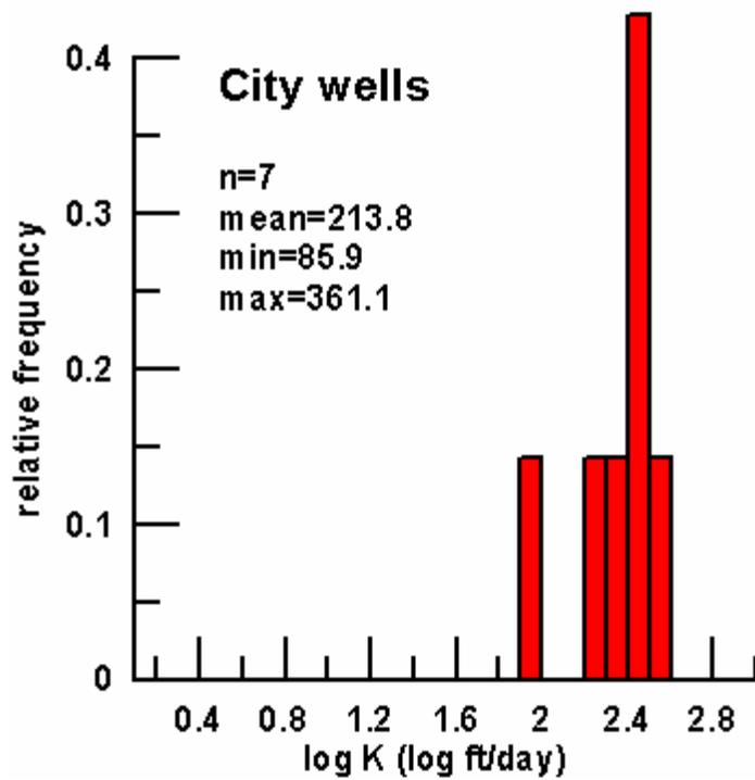
Figure 9. Histograms of results from hydraulic conductivity estimation using slug tests and pumping tests.
