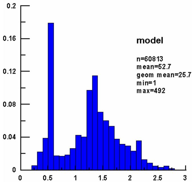
Figure 14. Comparison of field- and model-derived hydraulic conductivities for unlithified materials.
