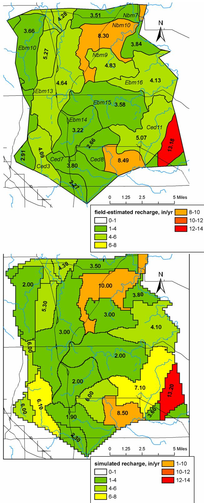
**Figure 11. Estimated recharge rates. Top: rates estimated by Cherkauer (2004). Bottom: rates determined through model calibration. Italicized abbreviations refer to surface-water basins.**
