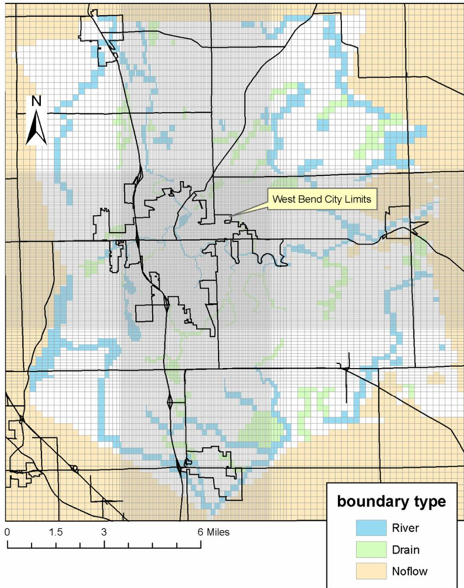
Figure 8. MODFLOW model grid and boundary conditions
