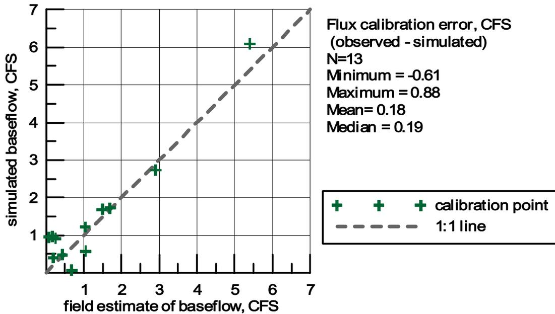
Figure 12. Model calibration results. Top: head calibration. Bottom: flux calibration.
