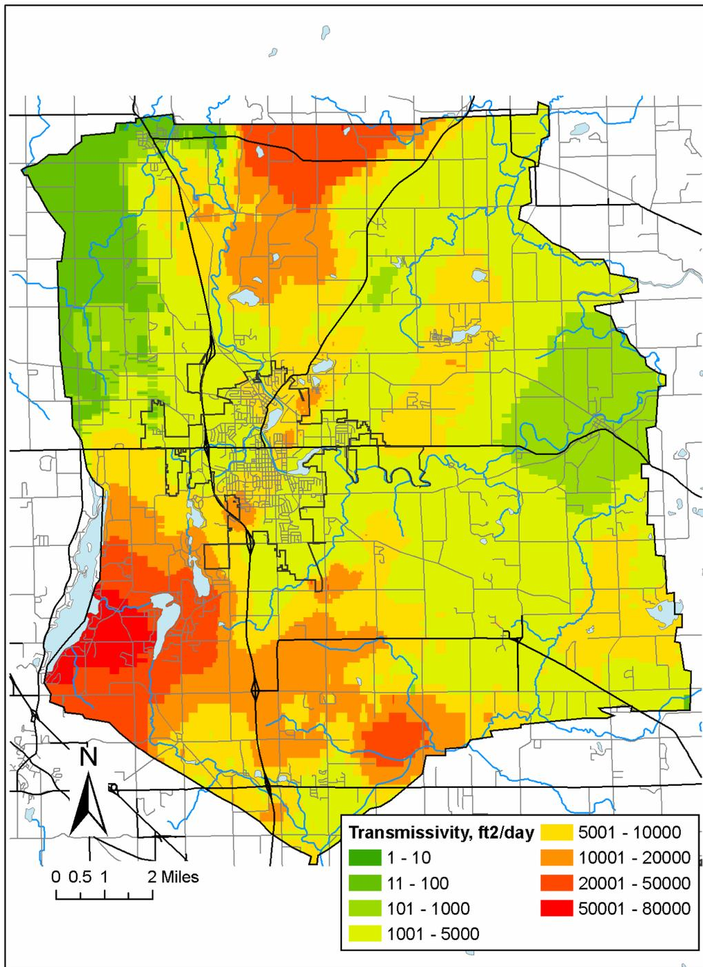
Figure 15. Transmissivity of the sand-and-gravel aquifer, based on model calibration.
