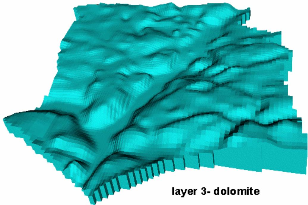
**Figure 6. Three-dimensional depiction of aquifer units represented by the model (model area shown on fig 1).**
