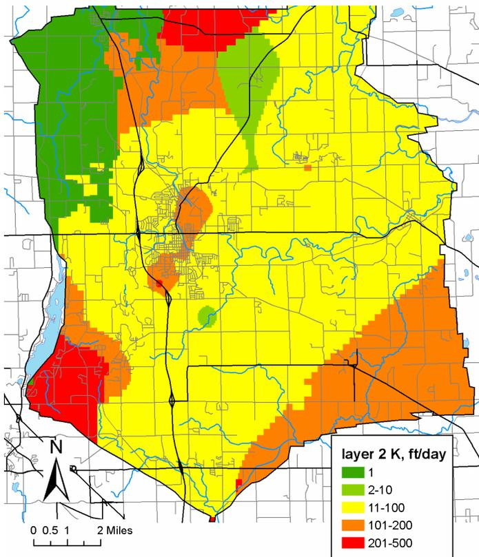
**Figure 13. Calibrated hydraulic conductivity distribution for model layers 1 (top) and 2 (bottom).**
