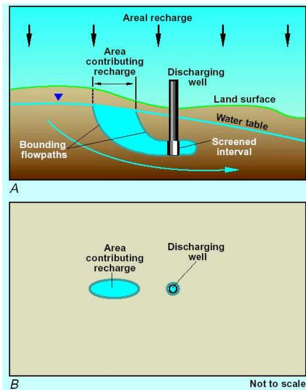
**Figure 18. Concepts of contributing area for a discharging well.** Top: zone of contribution terminology from USEPA (1987). Bottom, illustration of three-dimensional effects of a contributing area for a well (Focazio and others, 2002).
