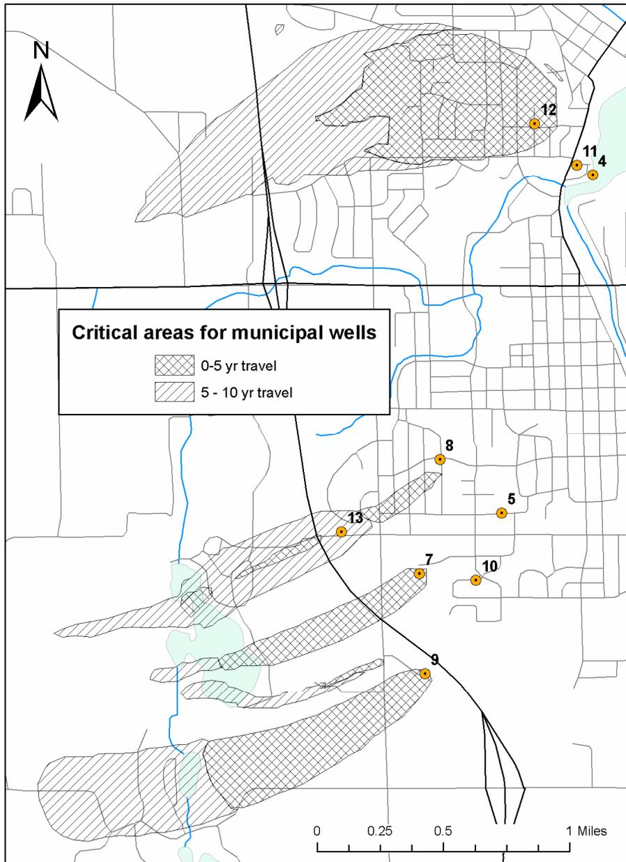
**Figure 20. Areas contributing surface water and/or infiltrating precipitation to West Bend municipal wells for 5- and 10-year times of travel.**
