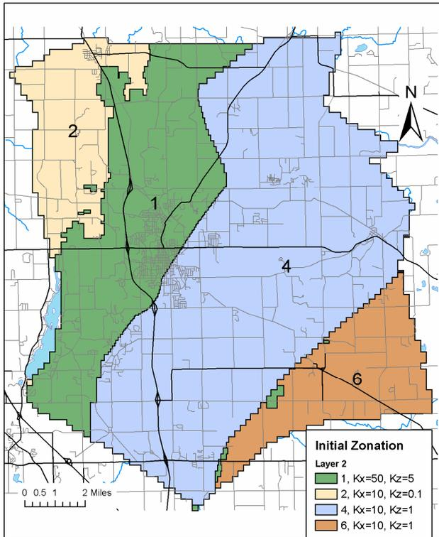
Figure 10. Initial hydraulic conductivity zonation for model layers 1 (top) and 2 (bottom).
