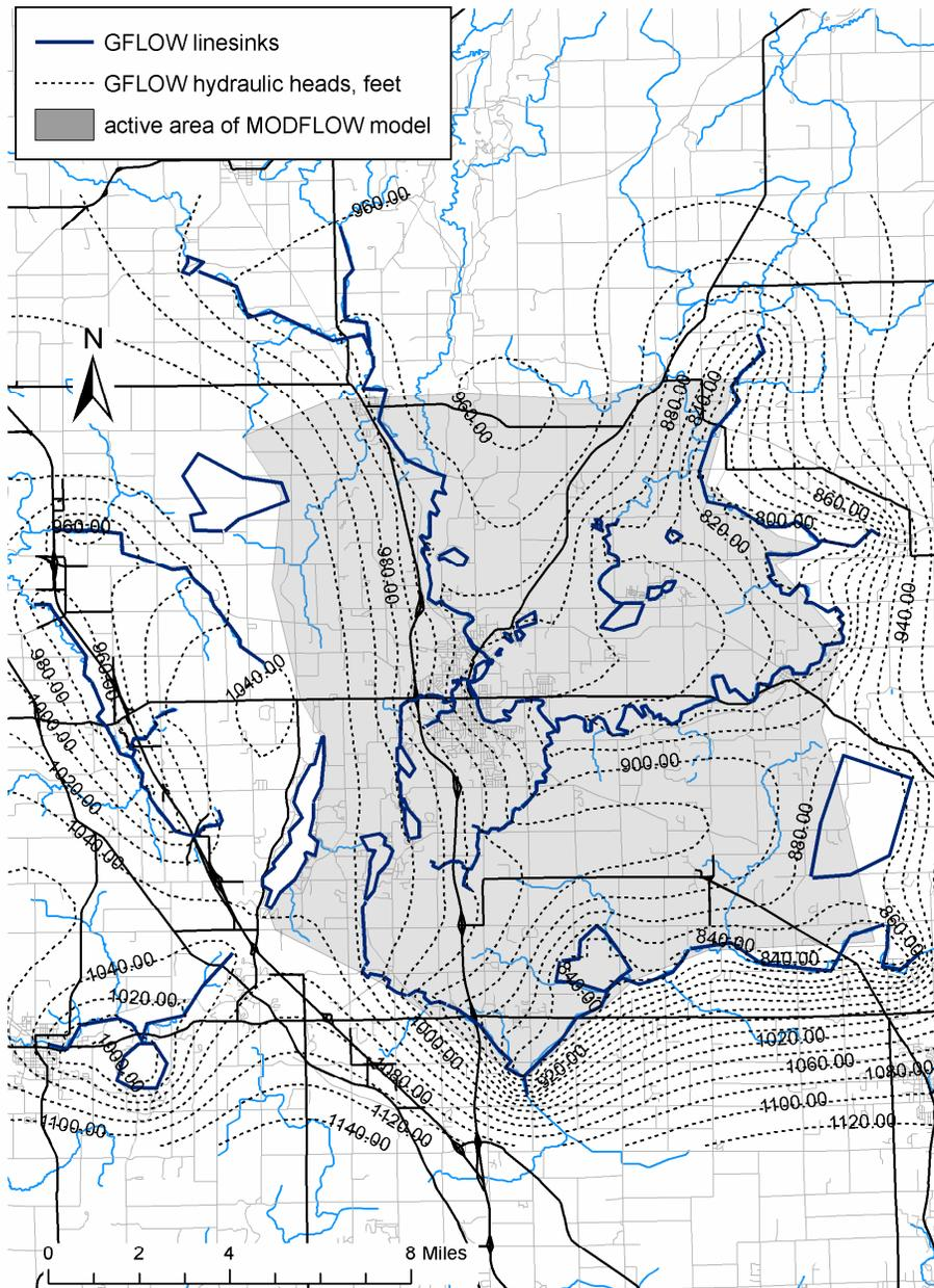
Figure A1. Extent of the GFLOW screening model developed for West Bend.
