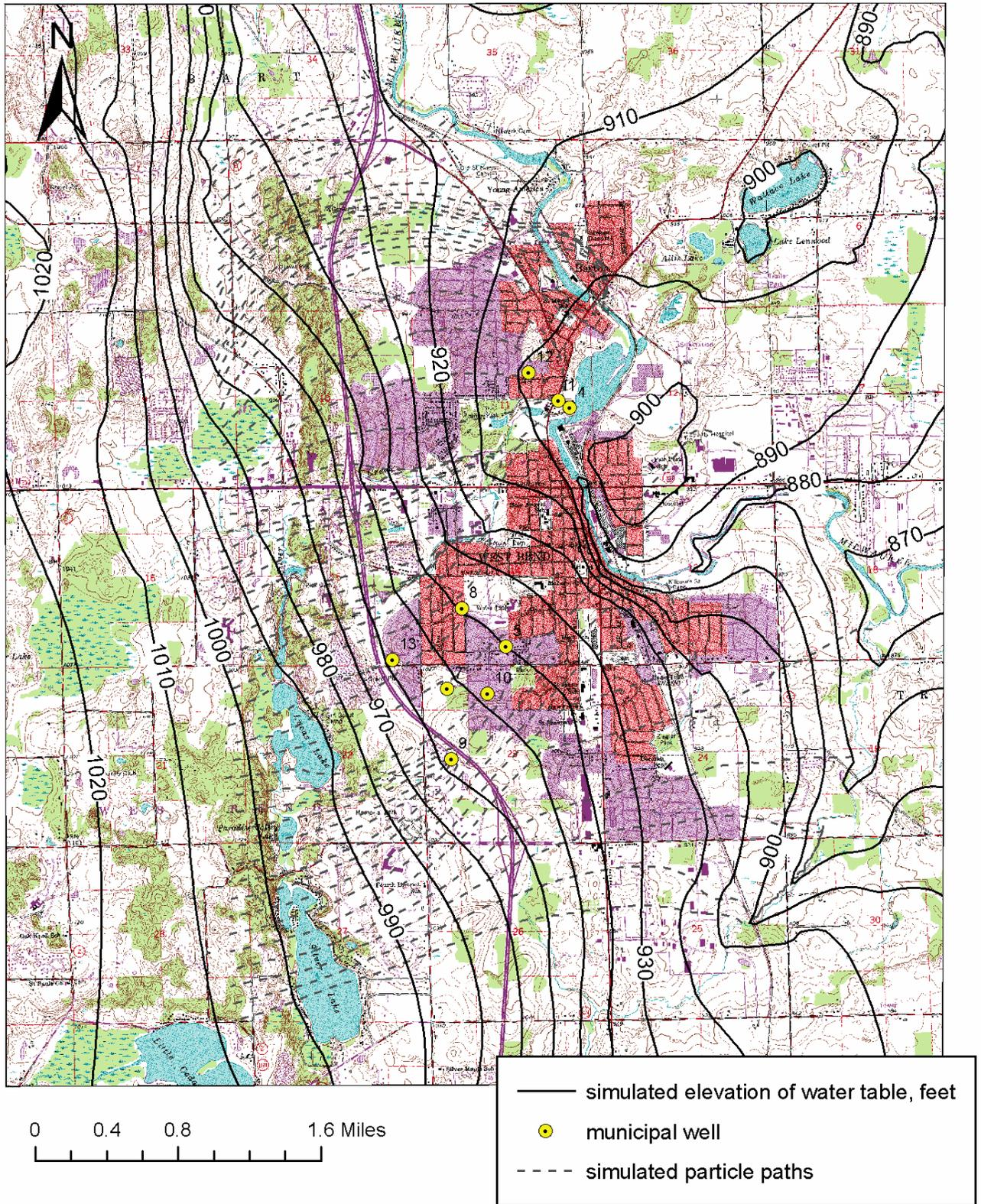
Figure 16. Simulated water table elevations and particle paths in the West Bend area.
