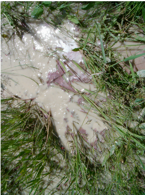
Figure 18. Cuttings showing ground-up packer.
