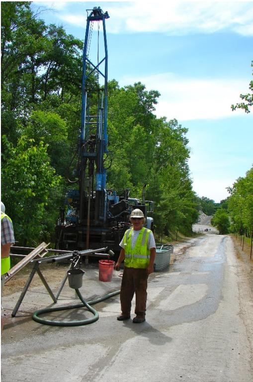
*Figure 16. WGNHS core drill rig in operation.*
