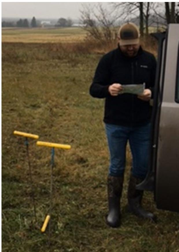
*Figure 12. Three push probes in area of shallow bedrock. The central probe is pushed into a vertical fracture. (Photo: David Hart).*
