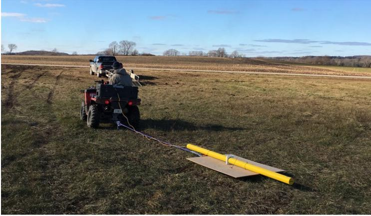
*Figure 14. A DualEM ground conductivity meter in use. This unit records both data and location at the same time. (Photo: David Hart.*
