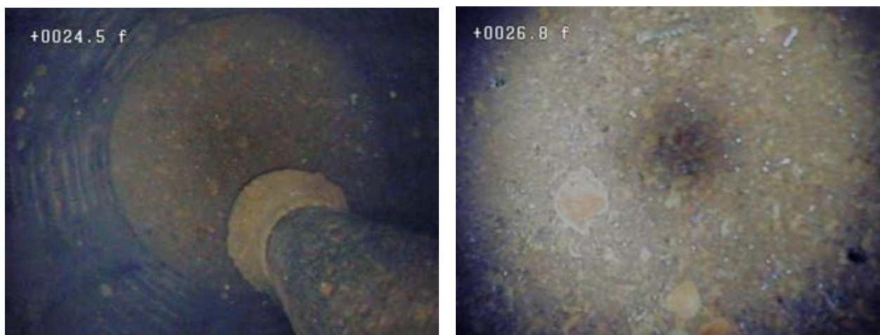
Figure 81. Still shots from borehole video taken May 8, 2020, in well TA-01, showing pump intake at base of well and slots in screen (left). Well bottom (right).
