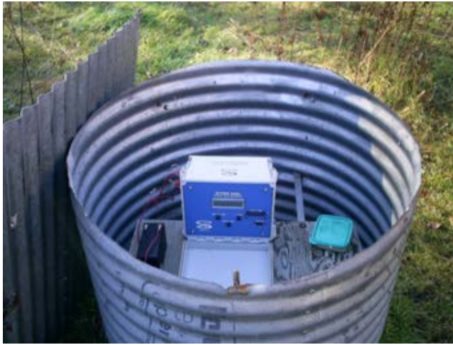
Figure 64: MO-02 well shelter and equipment before replacement (left) and old 3-in.-diameter PVC casing insert, exposed after shelter and equipment was removed (right). Photos courtesy of U.S. Geological Survey
