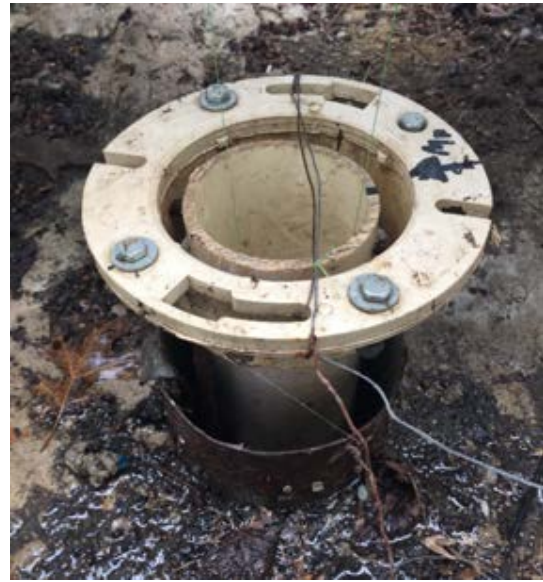
Figure 64: MO-02 well shelter and equipment before replacement (left) and old 3-in.-diameter PVC casing insert, exposed after shelter and equipment was removed (right). Photos courtesy of U.S. Geological Survey
