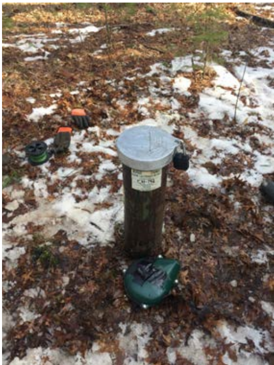
Figure 16. CH-142 well head with steel casing stick up and locking steel well head cap. Photos courtesy of U.S. Geological Survey.
