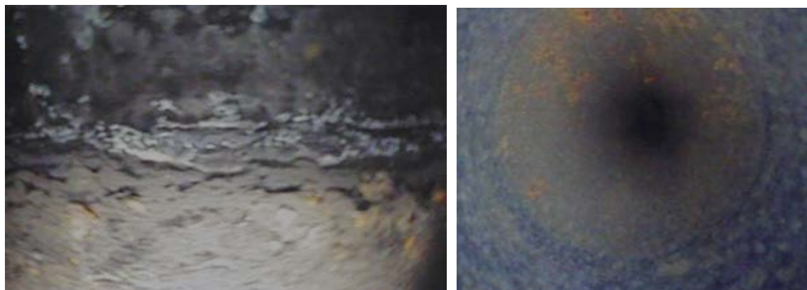
Figure 74. Still shots from borehole video log of MQ-09, collected December 4, 2019, showing bottom of casing, looking at the borehole wall, at 121 ft blsd (left) and bottom of well at 248.6 ft blsd looking directly down the borehole (right).
