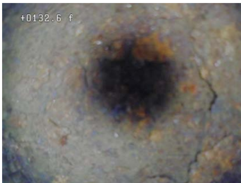
Figure 97. Still shot from borehole video log of WW-83 showing obstruction at about 133 ft bls, at which point the camera could not go any deeper.
