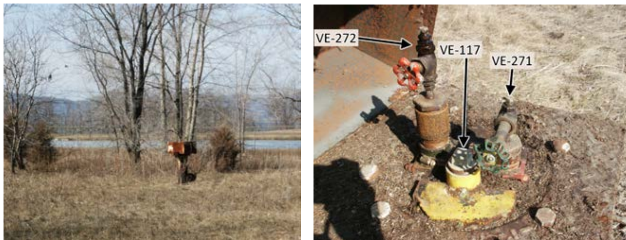
Figure 88. Monitoring shelter (left) and piezometer heads for VE-117, VE-271, and VE-272 (right) before work was completed. Work was completed from summer to winter 2019. Photo courtesy of U.S. Geological Survey.
