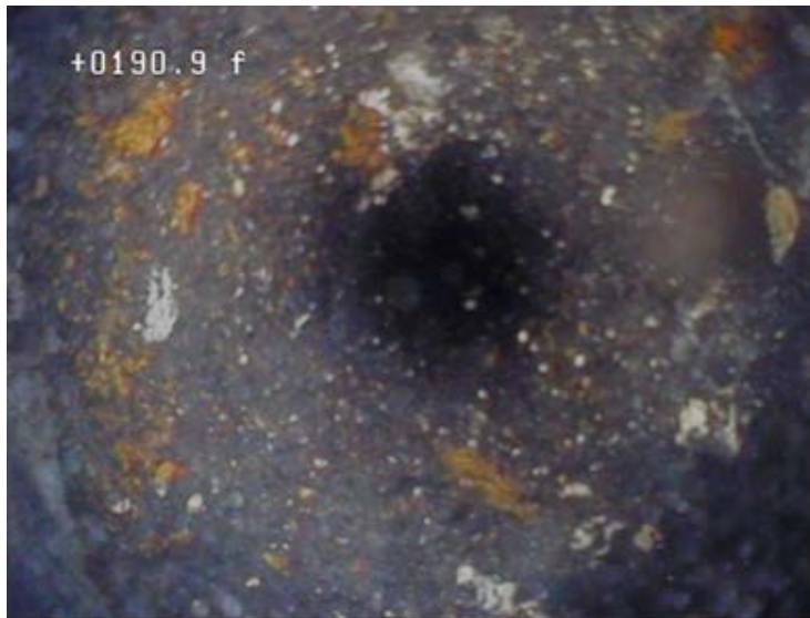
Figure 91. Still shots from borehole video log of WK-31 collected on December 18, 2018, showing the location of the blockage in the well at approximately 190 ft-BTOC as measured by the video equipment.
