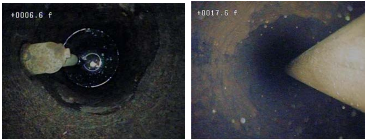
Figure 80. Still shots from borehole video taken May 8, 2020, in well TA-01, showing pit-less adapter and piping above water level (left) and deposits along the well's sidewall (right).
