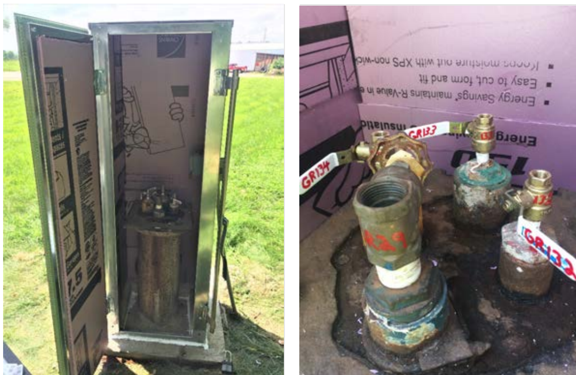
Figure 33. New insulated and heated well shelter (left) and piezometers GR132, GR-133, and GR-134 heads in the shelter (right). Work was completed in May of 2020. Photos courtesy of U.S. Geological Survey.
