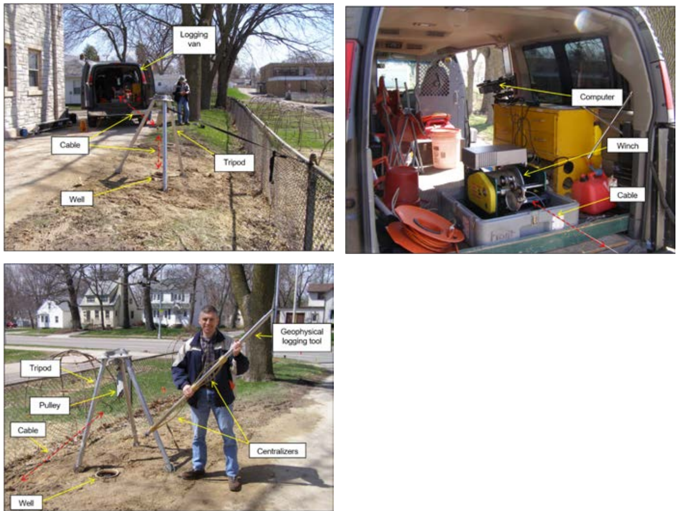
Figure 2. WGNHS borehole geophysics setup at a monitoring well. Top left photo shows the logging van with the fiber-optic cable running from the winch inside the logging van, to the tripod, and down to the borehole logging tool suspended within the well. Top right photo shows a more detailed view inside the logging van, where a live feed of borehole geophysical data can be viewed on the computer. Bottom photo shows the well head and centralizers, which stabilize certain geophysical logging tools at the center of the well during logging.
