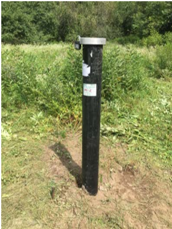
Figure 65. MO-02 with new protective steel well-head cover placed over the 5-in.-diameter casing. Work was completed in August of 2019. Photos courtesy of U.S. Geological Survey.
