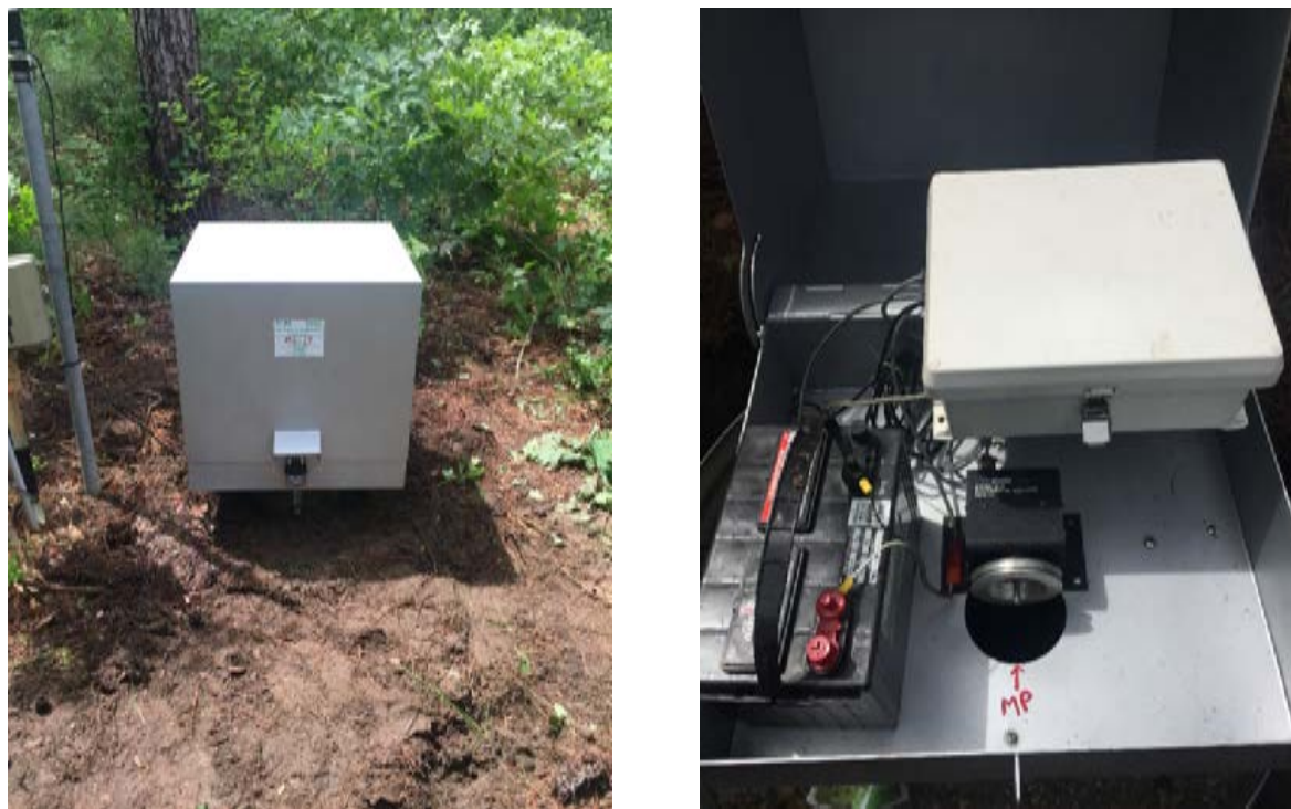
Figure 69: New flip-top well shelter (left) installed at MO-17. The shaft encoder was reinstalled when the flip-top shelter was installed in summer 2019 but eventually replaced with a pressure transducer (right) in January 2020. Photos courtesy of U.S. Geological Survey.
