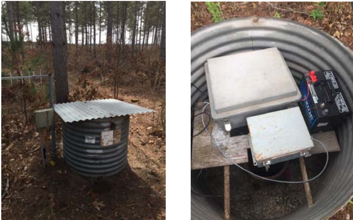
Figure 68: MO-17 galvanized well shelter (left) with shelf holding shafter encoder and float (right), before replacement. Photos courtesy of U.S. Geological Survey.
