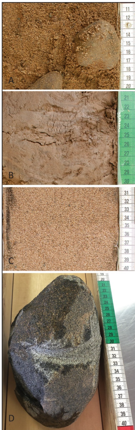
Figure 5. Photos of typical sediment types in core RS1 with interpreted depositional environment for these sediment types: (panel A) sand and gravel (stream sediment), (panel B) laminated silty clay (lake sediment), (panel C) sand (stream sediment), and (panel D) rock ground by the core bit, which may create gray dust in samples. Measuring tape in cm for scale.
